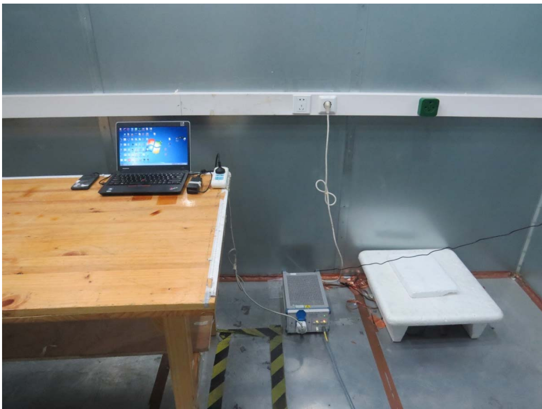
Picture 3 Conducted Emission Test Setup
