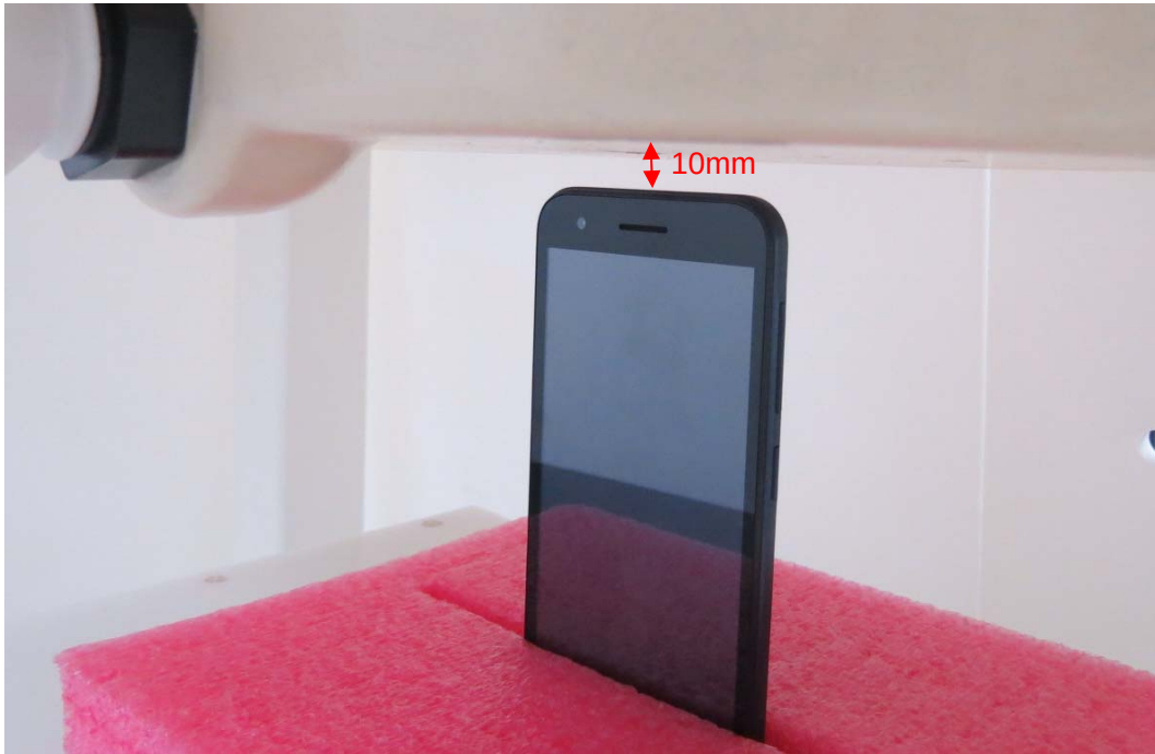
Top Side, the distance from handset to the bottom of the Phantom is 10mm
