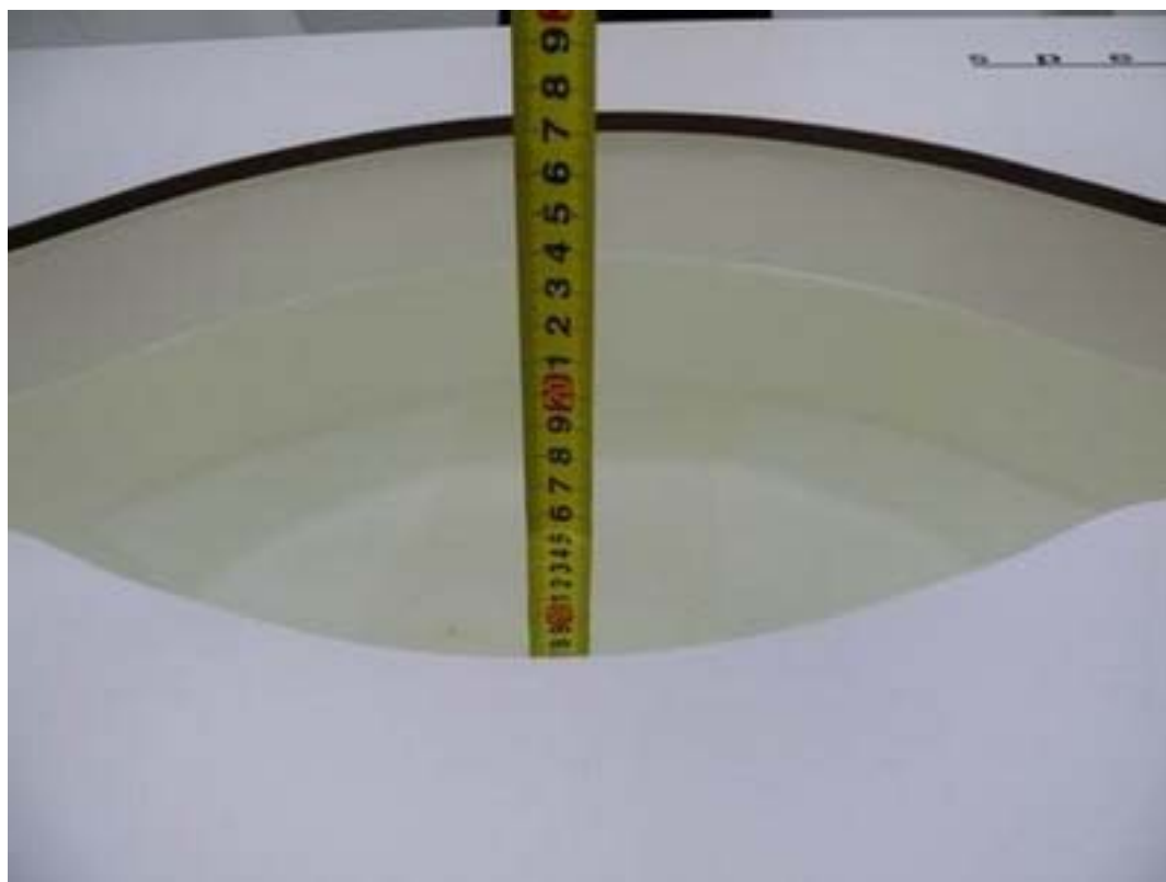
Picture 10: Liquid depth in the flat Phantom (2600 MHz, 15.3cm depth)
