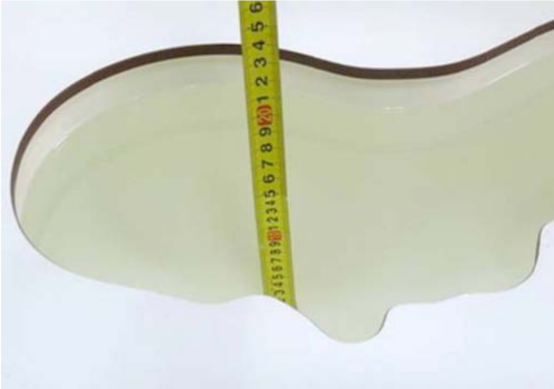
Picture 5: liquid depth in the head Phantom (1900 MHz, 15.3cm depth)
