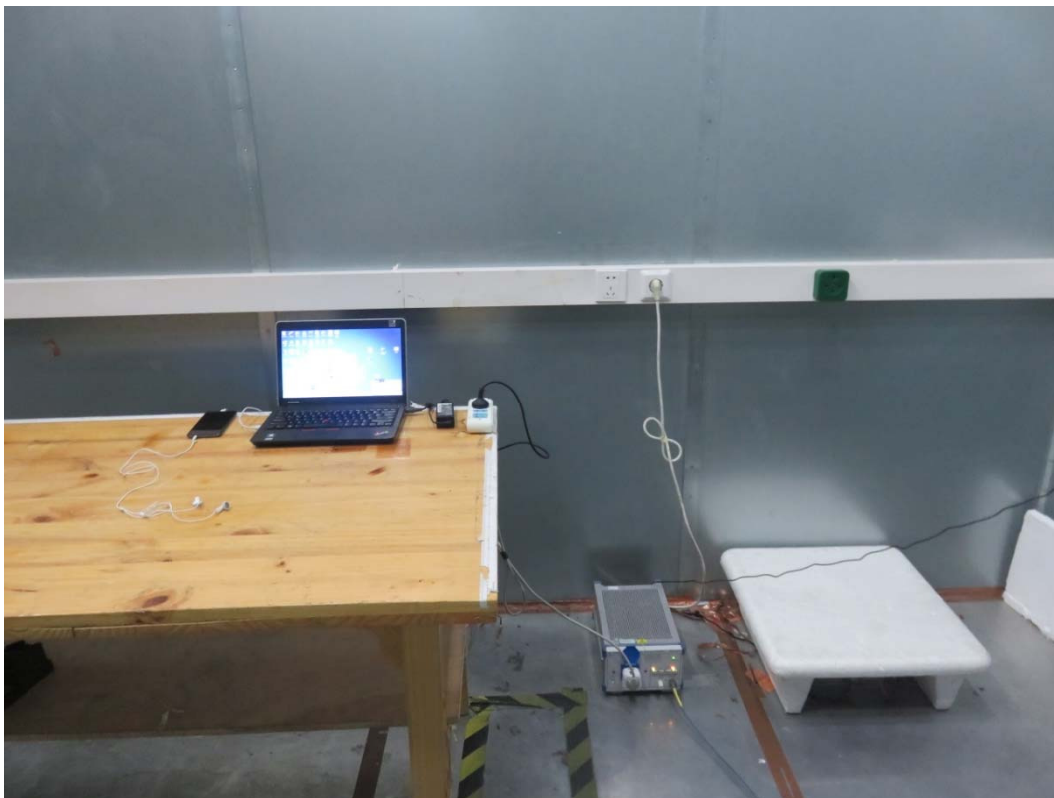
Picture 3 Conducted Emission Test Setup
