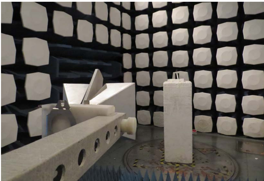
Picture 2: Radiated Spurious Emissions Test setup
