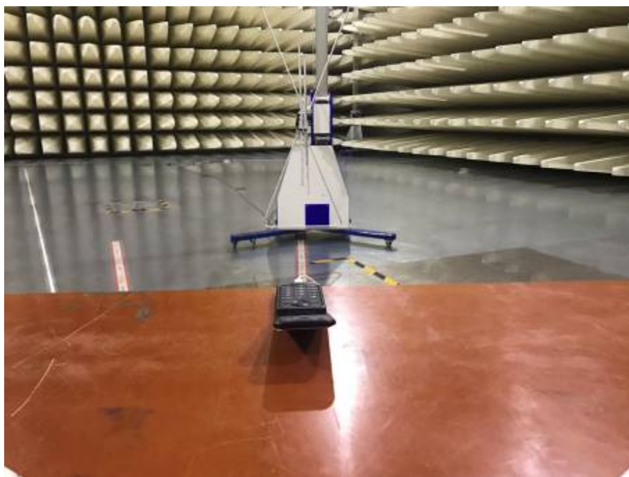
Radiated Emissions Test Setup (with charger) (30-1000MHz)
