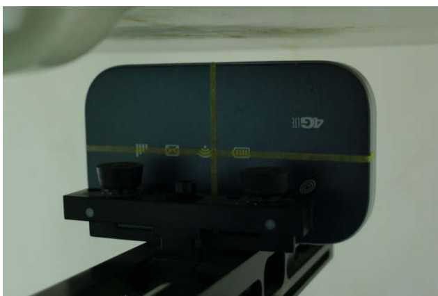
Bottom Side of the DUT with Phantom 10 mm Gap
