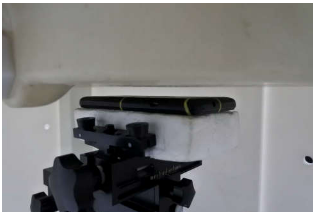
Back, Test Separation 10 mm
