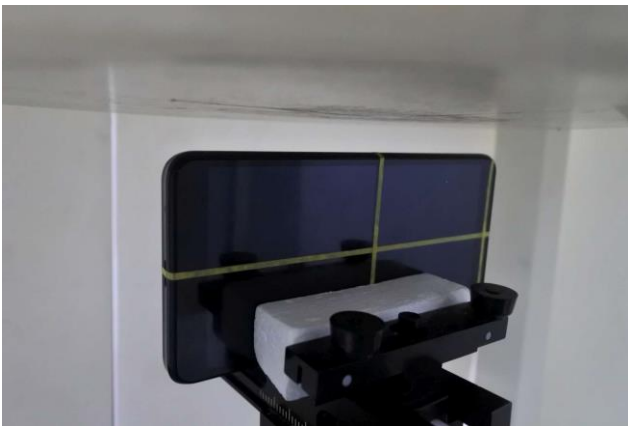
Left Side, Test Separation 10 mm
