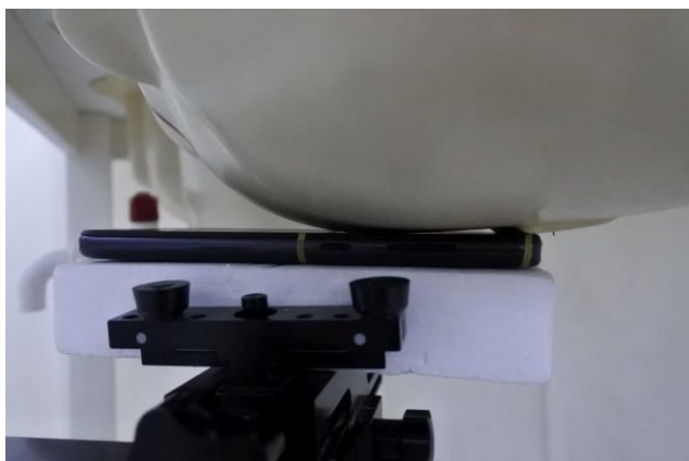
Left Cheek, Test Separation 0 mm
