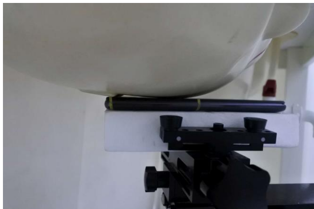
Right Cheek ,Test Separation 0 mm
