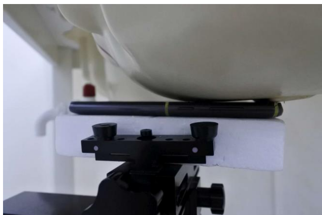
Left Cheek, Test Separation 0 mm
