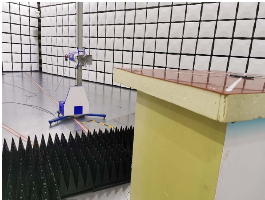
Spurious Radiated Emissions Test setup
