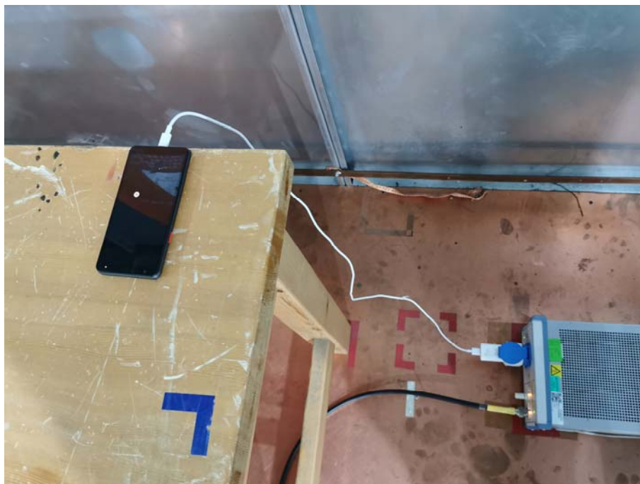
Conducted Emissions Test Setup (with charger)
