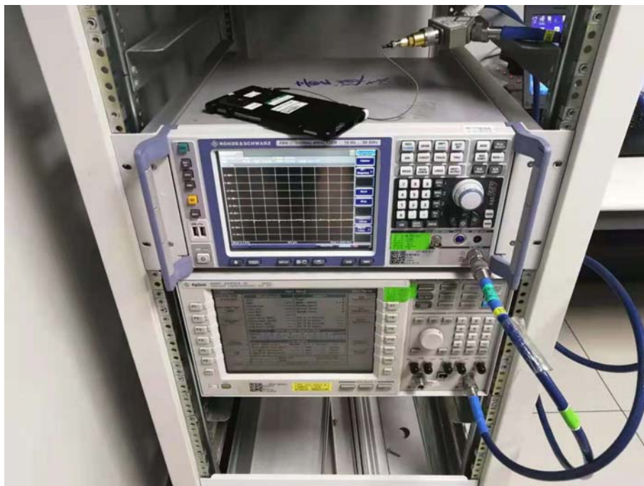
RF Conducted Test setup (GSM/WCDMA/LTE)
