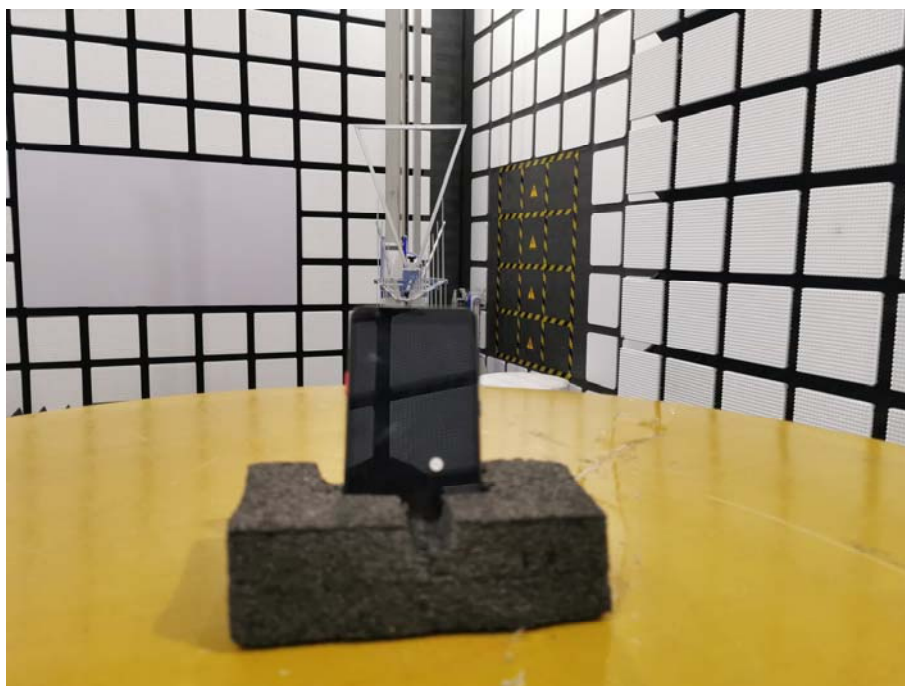
Spurious Radiated Emissions Test setup
