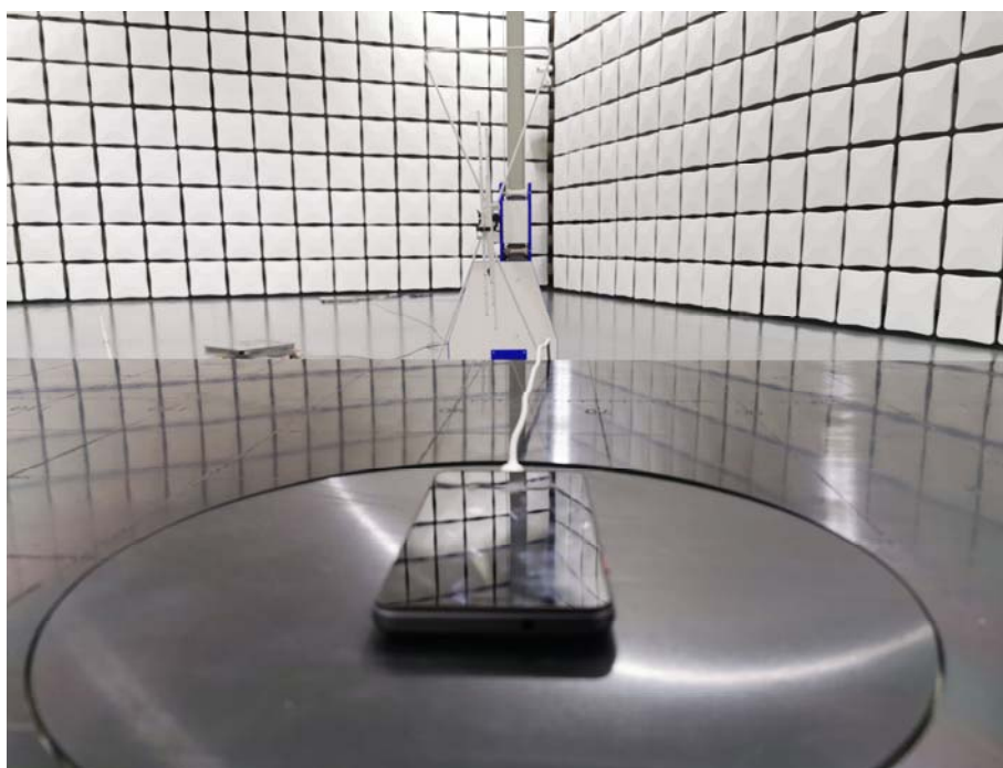
Spurious Radiated Emissions Test setup
