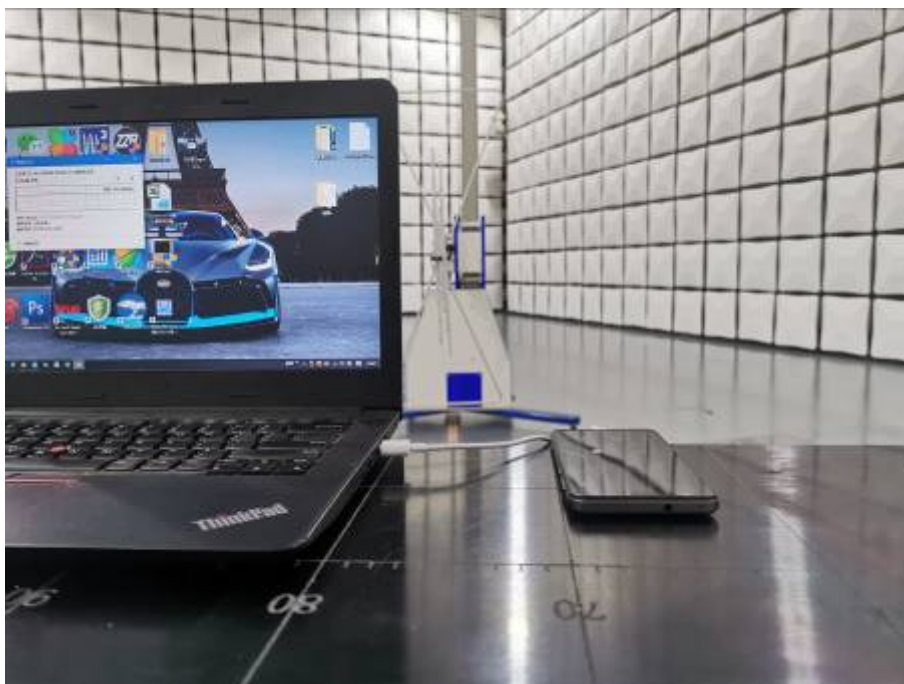
Radiated Emissions Test Setup (with laptop) (30-1000MHz)
