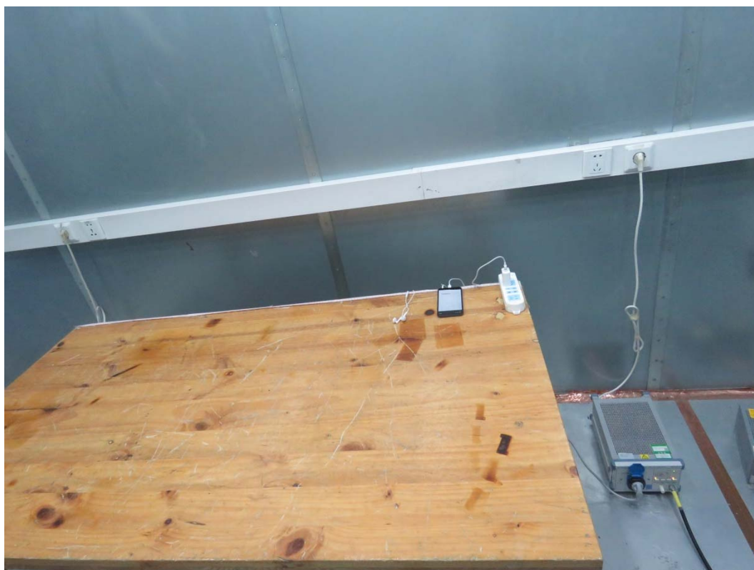
Picture 2 Conducted Emission Test Setup
