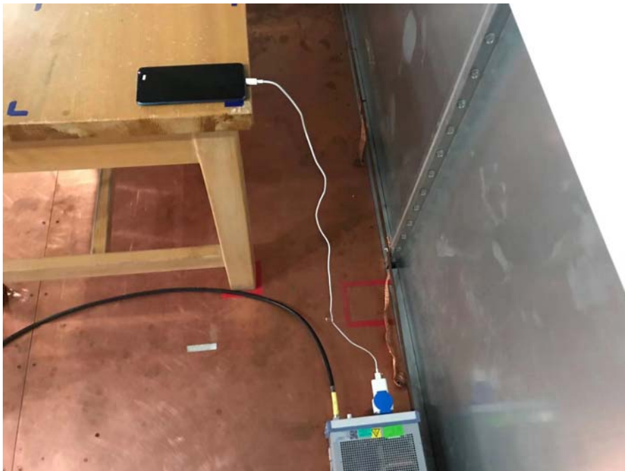
Conducted Emissions Test Setup (with charger)
