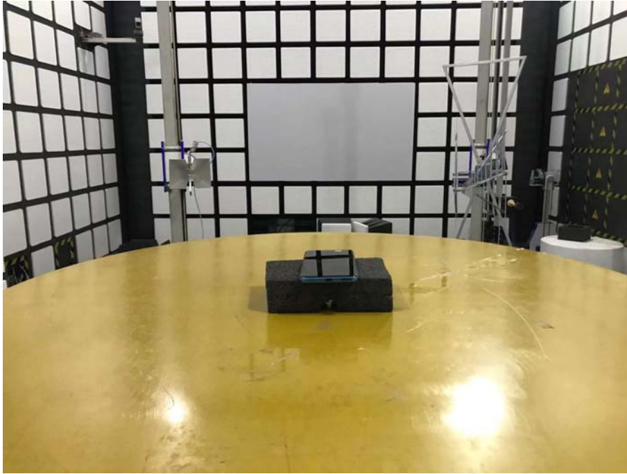
Spurious Radiated Emissions Test setup
