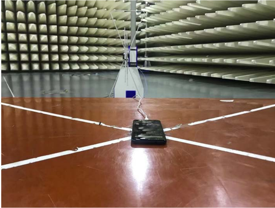
Spurious Radiated Emissions Test setup
