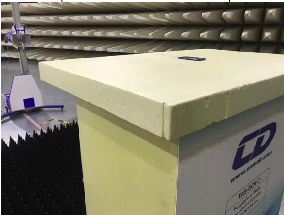
Spurious Radiated Emissions Test setup
