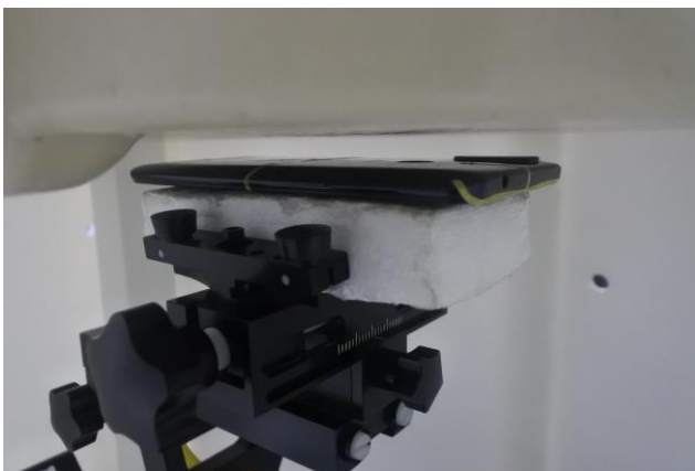
Back, Test Separation 10 mm
