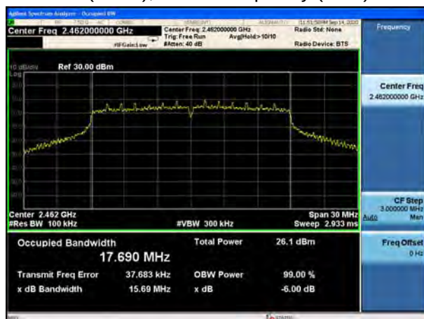
802.11n(HT20), Carrier frequency (MHz): 2462
