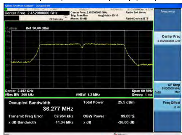
802.11n(HT40), Carrier frequency (MHz): 2452
