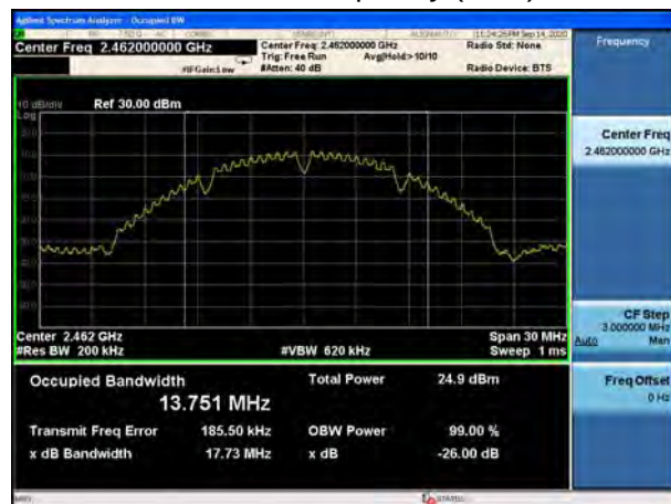
802.11b, Carrier frequency (MHz): 2462
