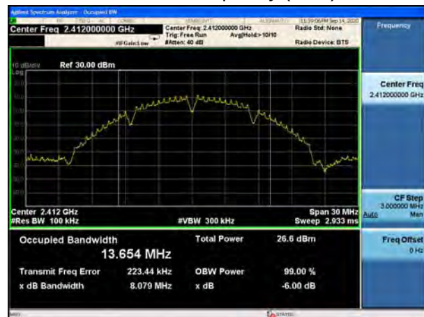
802.11b, Carrier frequency (MHz): 2437
