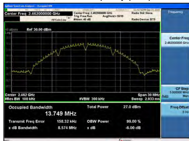
802.11b, Carrier frequency (MHz): 2462
