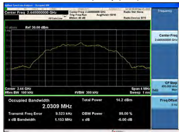
BLE-2M Carrier frequency (MHz): 2480
