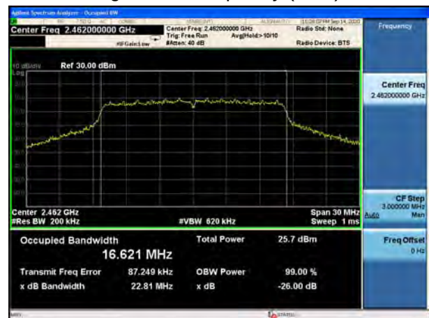
802.11g, Carrier frequency (MHz): 2462
