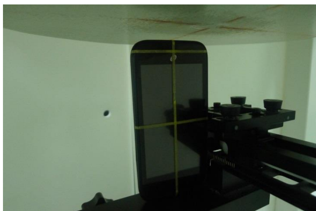
Top Side, Test Separation 10 mm
