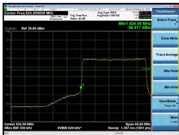
DC_2A_n5A 256QAM 20MHz CH-Low 100%RB
