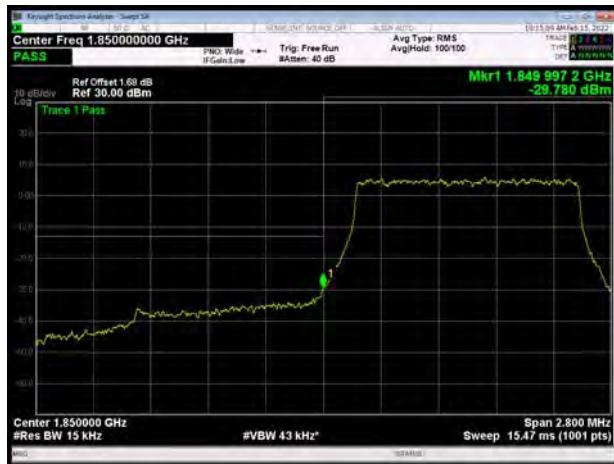
LTE Band 2 3MHz QPSK 1RB CH-Low
