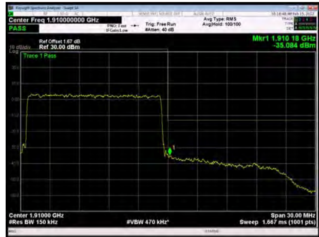
LTE Band 2 20MHz 16QAM 1RB CH-High
