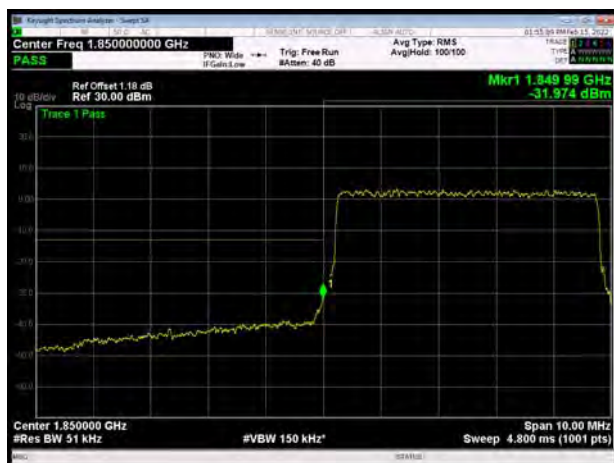
LTE Band 2 5MHz 64QAM 100%RB CH-Low
