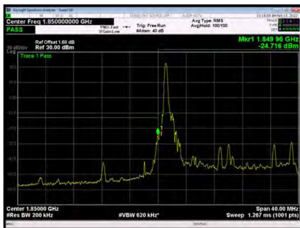
LTE Band 2 20MHz QPSK 100%RB CH-Low
