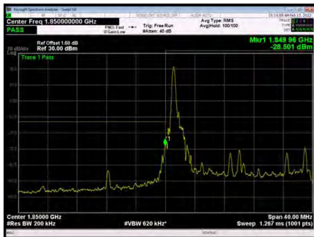
LTE Band 2 20MHz 16QAM 100%RB CH-Low
