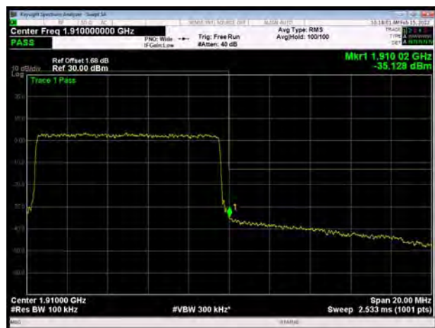
LTE Band 2 15MHz 16QAM 1RB CH-High
