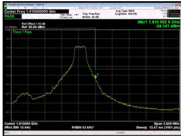
LTE Band 2 1.4MHz 64QAM 100%RB CH-High
