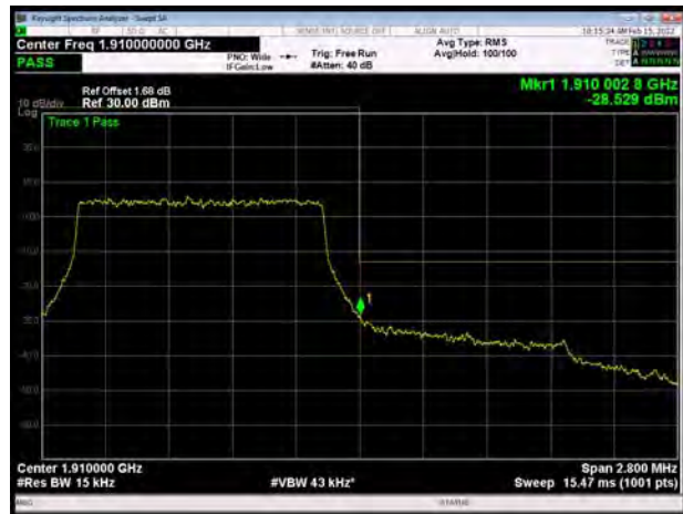
LTE Band 2 3MHz QPSK 1RB CH-High
