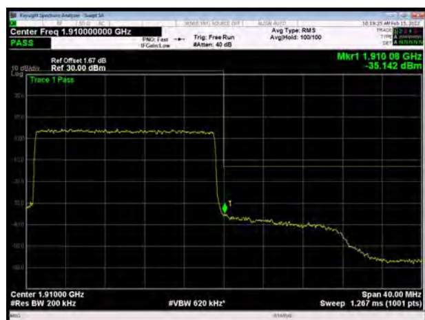
LTE Band 2 20MHz QPSK 100%RB CH-High
