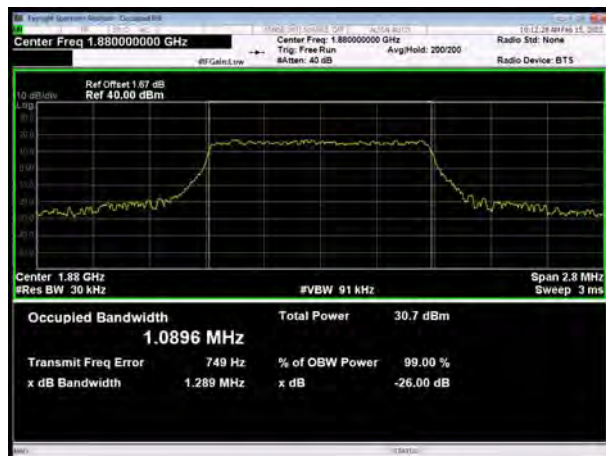
LTE Band 2 1.4MHz QPSK CH-High
