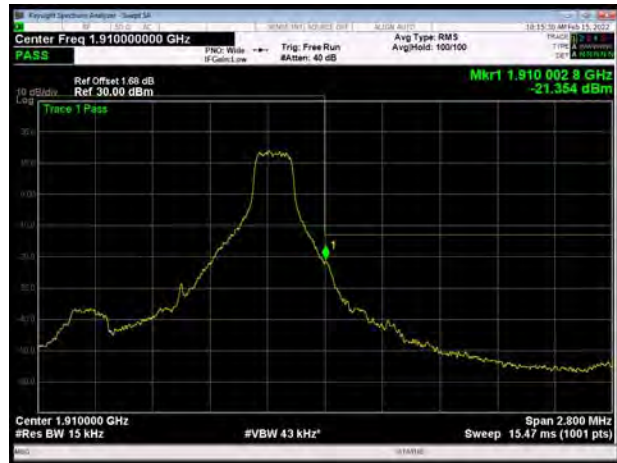
LTE Band 2 1.4MHz QPSK 100%RB CH-High
