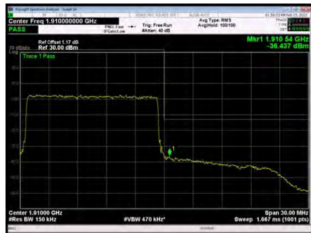
LTE Band 2 20MHz 64QAM 1RB CH-High
