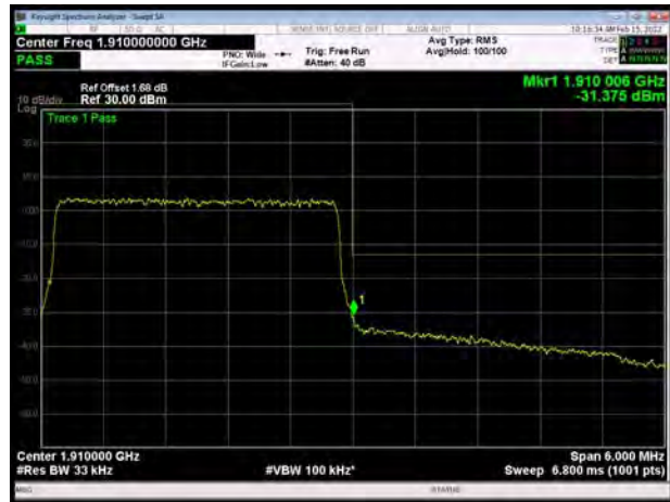
LTE Band 2 5MHz 16QAM 1RB CH-High
