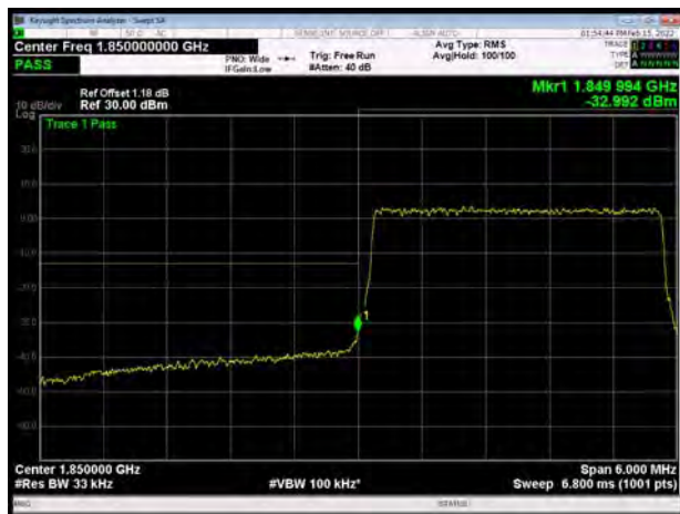
LTE Band 2 5MHz 64QAM 1RB CH-Low
