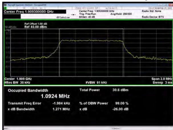
LTE Band 2 1.4MHz QPSK CH-High
