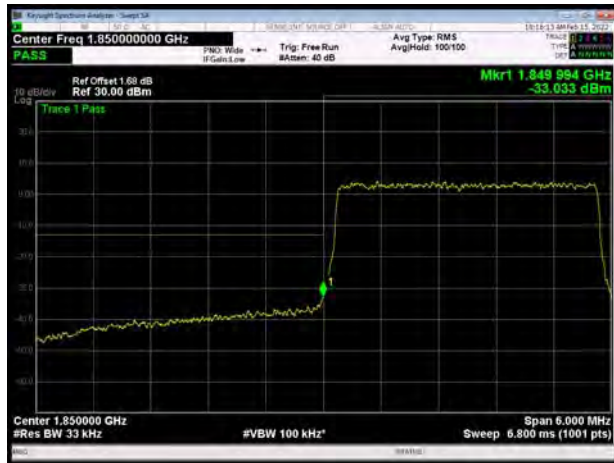
LTE Band 2 5MHz 16QAM 1RB CH-Low
