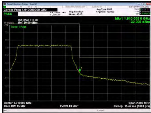
LTE Band 2 3MHz 64QAM 1RB CH-High
