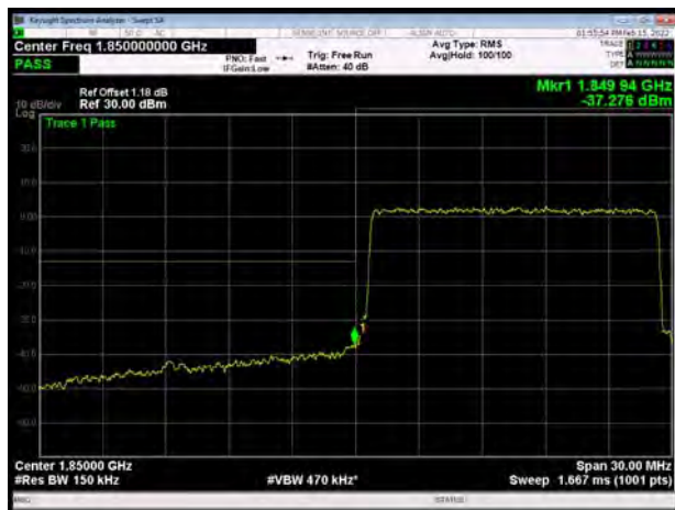
LTE Band 2 20MHz 64QAM 1RB CH-Low
