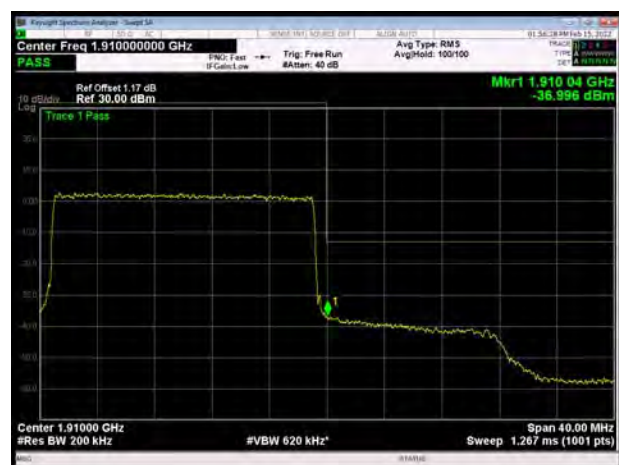
LTE Band 2 20MHz 64QAM 100%RB CH-High
