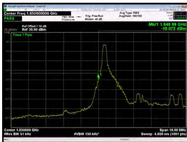
LTE Band 2 5MHz 64QAM 100%RB CH-Low
