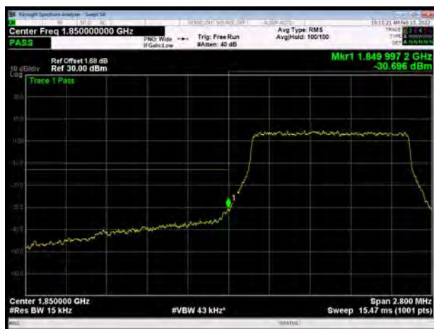
LTE Band 2 3MHz 16QAM 1RB CH-Low
