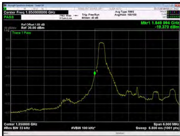
LTE Band 2 3MHz QPSK 1RB CH-Low
