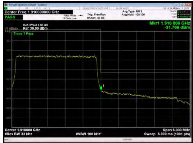
LTE Band 2 5MHz QPSK 1RB CH-High
