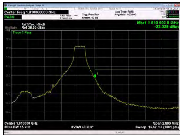
LTE Band 2 1.4MHz 16QAM 100%RB CH-High
