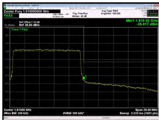
LTE Band 2 15MHz 64QAM 1RB CH-High
