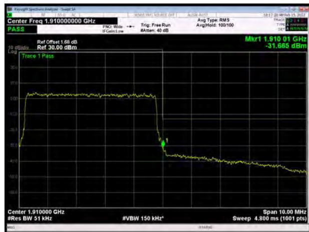
LTE Band 2 5MHz 16QAM 100%RB CH-High
