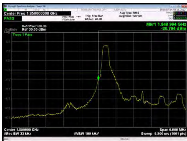
LTE Band 2 3MHz 16QAM 1RB CH-Low
