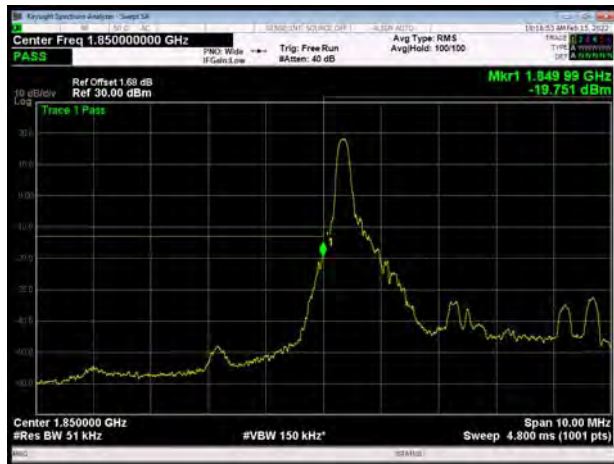
LTE Band 2 5MHz 16QAM 100%RB CH-Low
