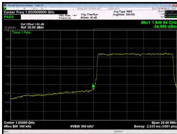
LTE Band 2 15MHz QPSK 1RB CH-Low
