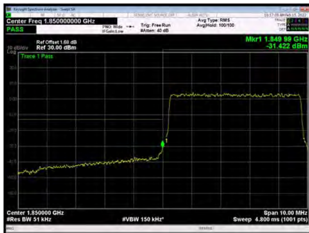
LTE Band 2 5MHz 16QAM 100%RB CH-Low
