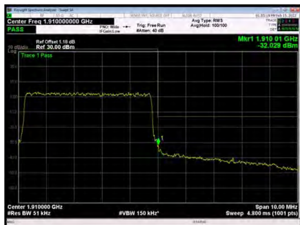
LTE Band 2 5MHz 64QAM 100%RB CH-High
