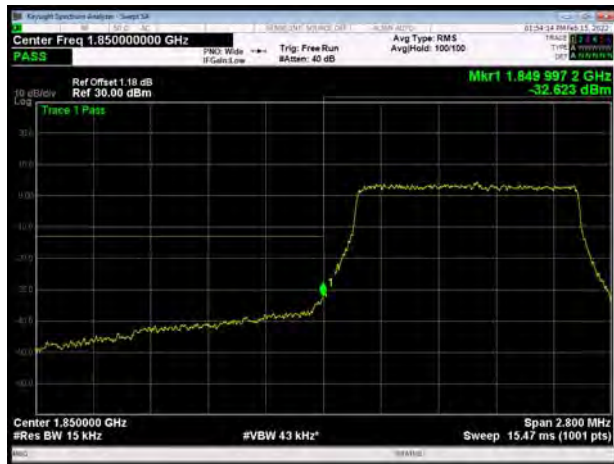
LTE Band 2 3MHz 64QAM 1RB CH-Low
