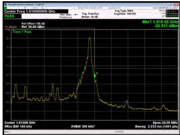
LTE Band 2 10MHz QPSK 100%RB CH-High
