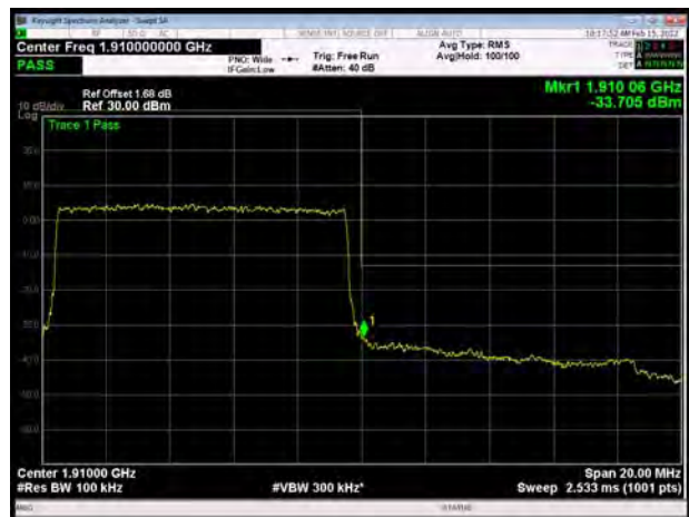
LTE Band 2 15MHz QPSK 1RB CH-High
