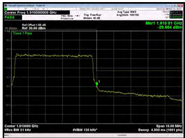
LTE Band 2 5MHz QPSK 100%RB CH-High
