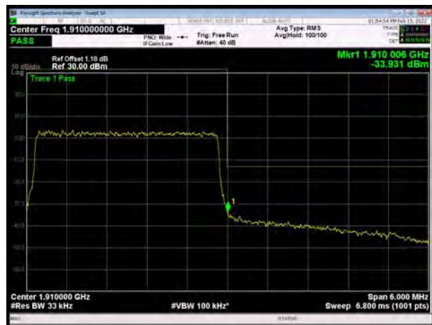
LTE Band 2 5MHz 64QAM 1RB CH-High
