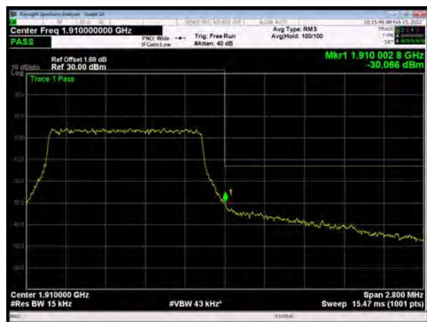
LTE Band 2 3MHz 16QAM 1RB CH-High
