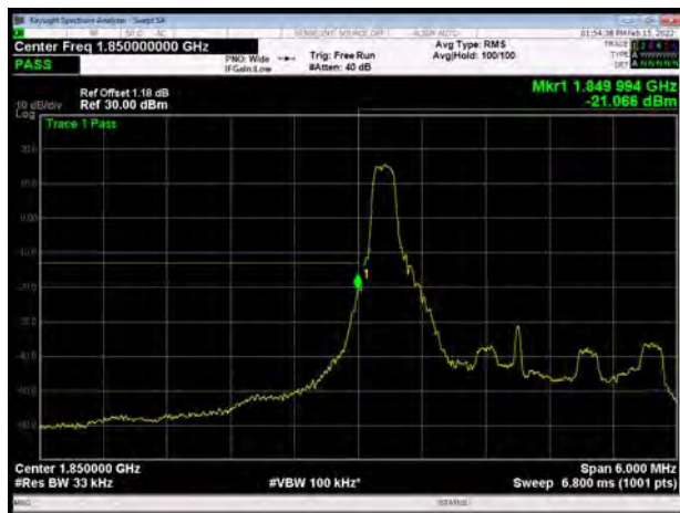
LTE Band 2 3MHz 64QAM 1RB CH-Low
