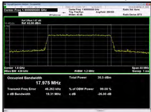
LTE Band 2 20MHz QPSK CH-High
