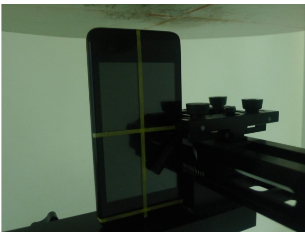
Bottom Side, Test Separation 1 cm
