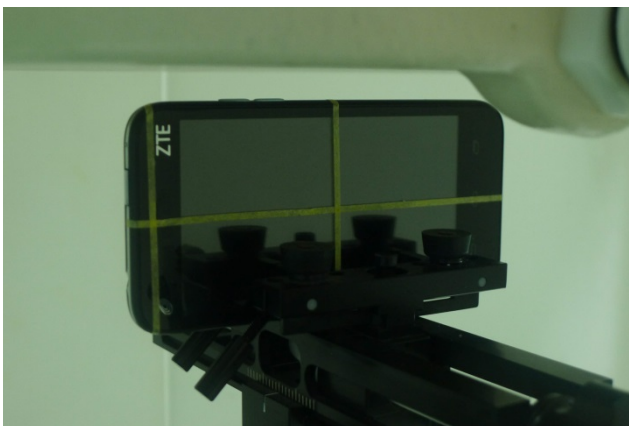
Right Side, Test Separation 1 cm
