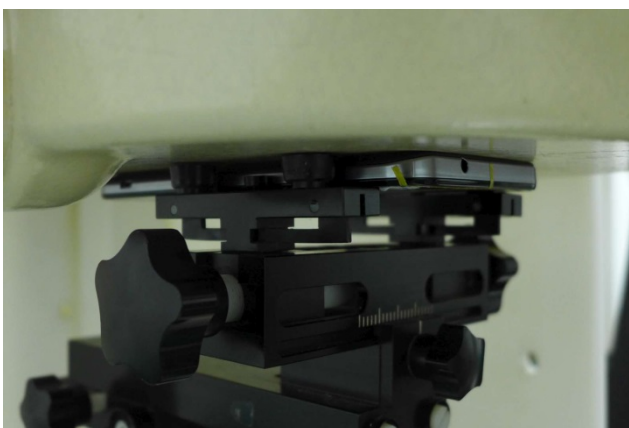
Back, Test Separation 0 cm (Extremity SAR)
