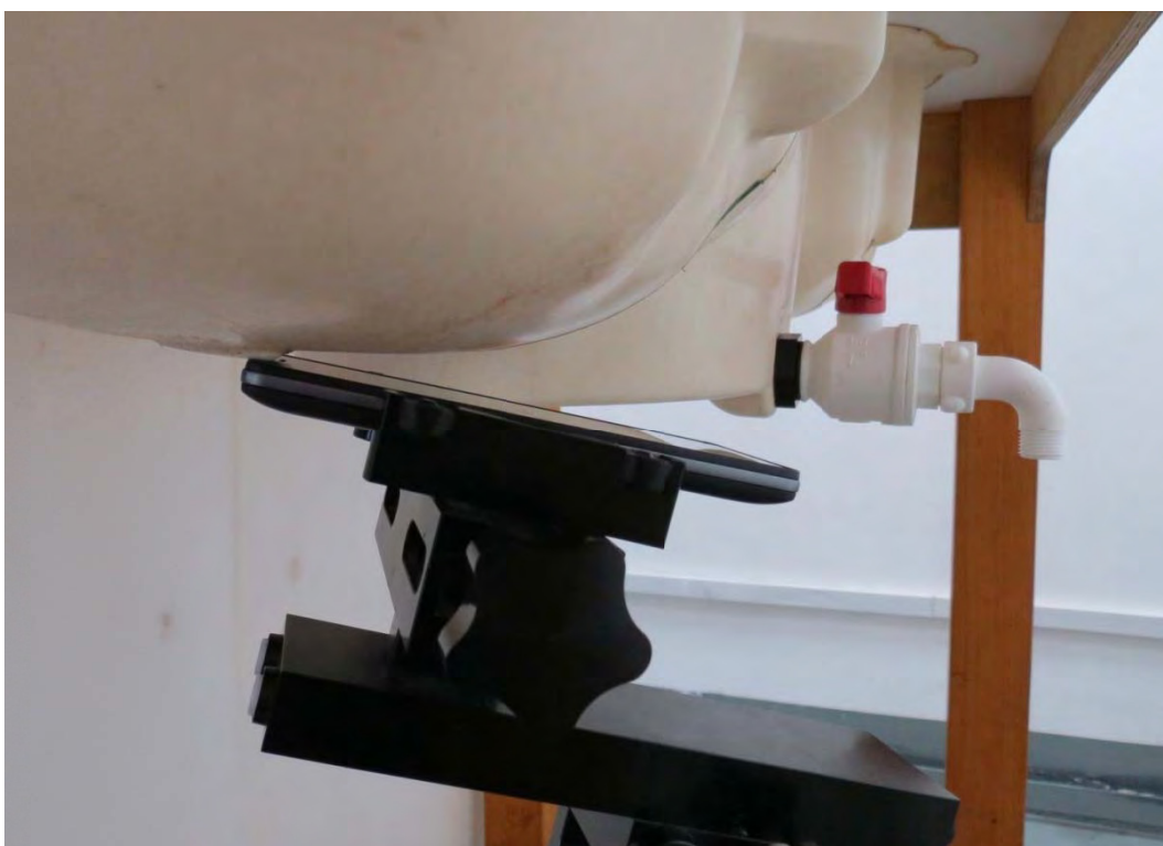
Picture 17: Right Hand Tilt 15 Degree Position Z815 (RXC1512-0230SAR01R1)
