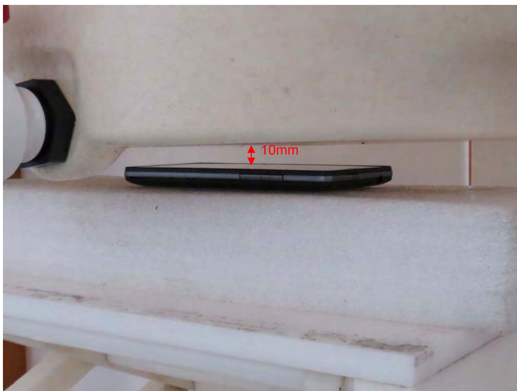
Picture 27: Front Side, the distance from handset to the bottom of the Phantom is 10mm Z815 (RXA1611-0257SAR)
