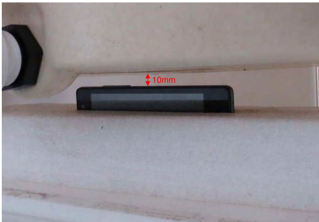
Picture 28: Right Side, the distance from handset to the bottom of the Phantom is 10mm Z815 (RXA1611-0257SAR)
