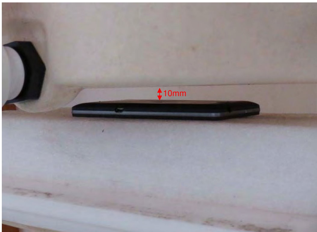
Picture 26: Back Side, the distance from handset to the bottom of the Phantom is 10mm Z815 (RXA1611-0257SAR)
