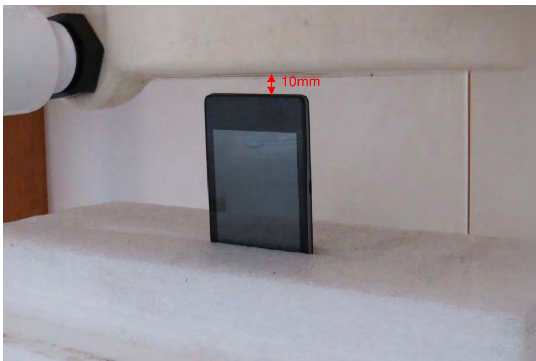
Picture 23: Bottom Side, the distance from handset to the bottom of the Phantom is 10mm Z815 (RXC1512-0230SAR01R1)
