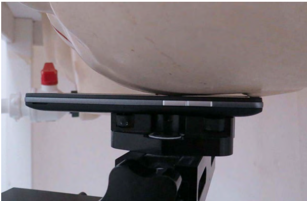
Picture 24: Left Hand Touch Cheek Position Z815 (RXA1611-0257SAR01R2)/ Z815 (RXA1707-0217SAR)
