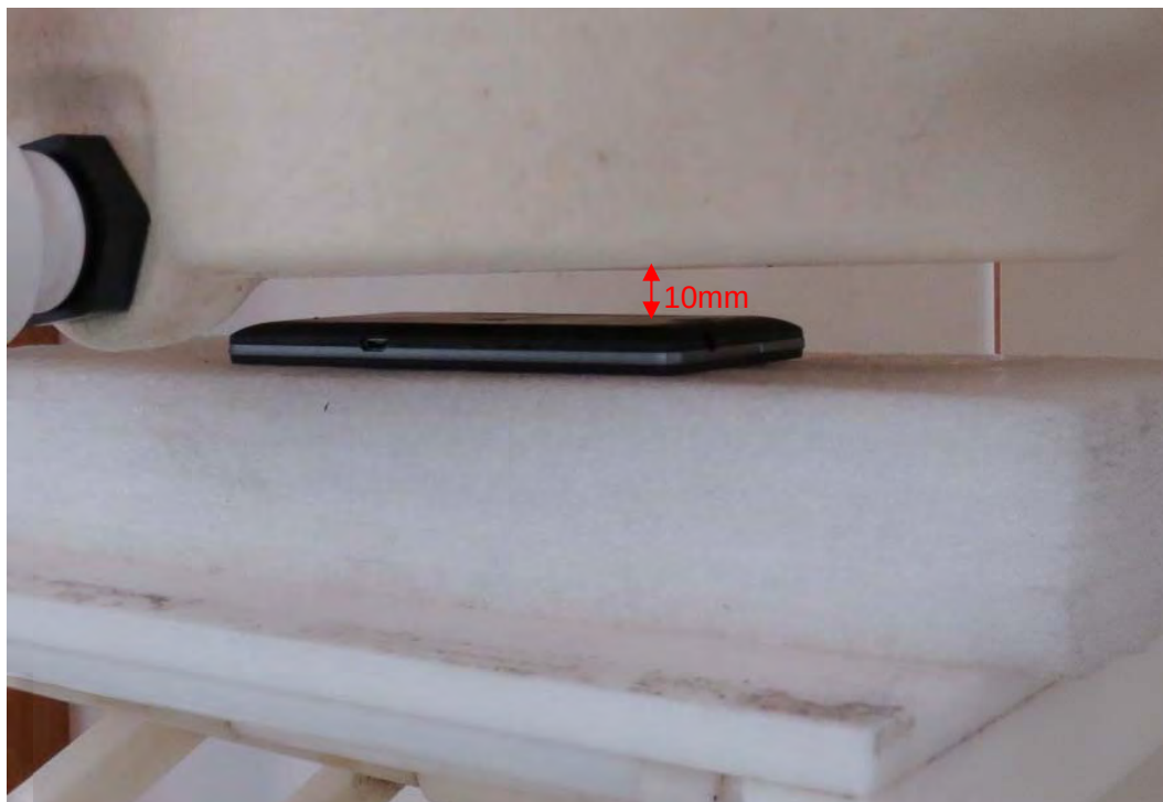
Picture 18: Back Side, the distance from handset to the bottom of the Phantom is 10mm Z815 (RXC1512-0230SAR01R1)
