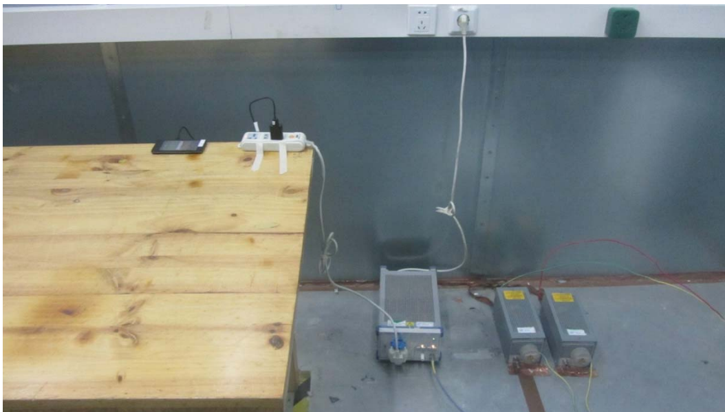
Picture 3 Conducted Emission Test Setup
