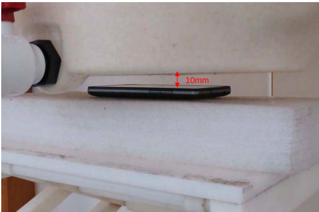
Picture 19: Front Side, the distance from handset to the bottom of the Phantom is 10mm
