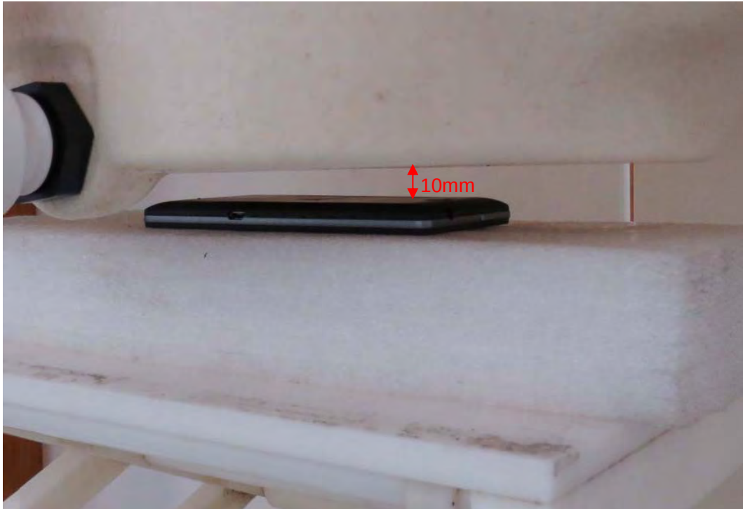
Picture 18: Back Side, the distance from handset to the bottom of the Phantom is 10mm
