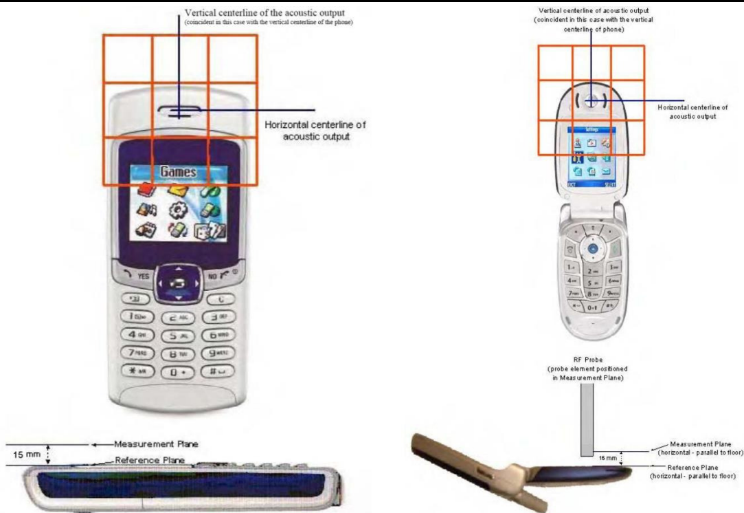
Fig 8.2 EUT reference and plane for HAC RF emission measurements
