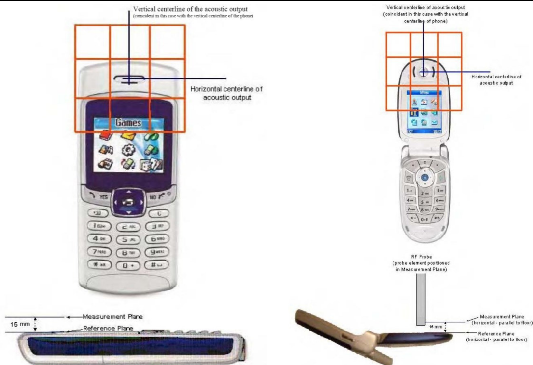
Fig 8.2 EUT reference and plane for HAC RF emission measurements
