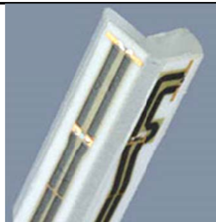
Fig 5.2 Photo of E-field Probe
