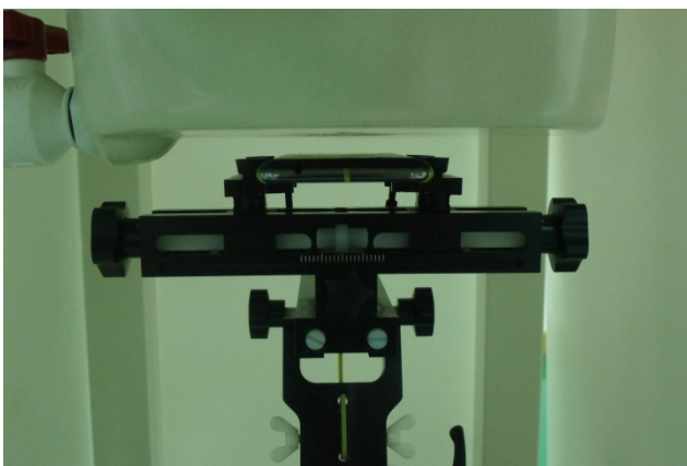
Back, Test Separation 1 cm
