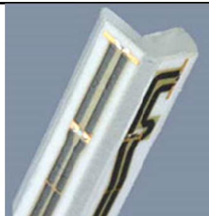
Fig 5.2 Photo of E-field Probe
