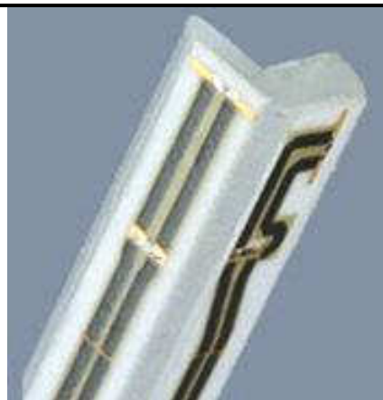
Fig 5.2 Photo of E-field Probe
