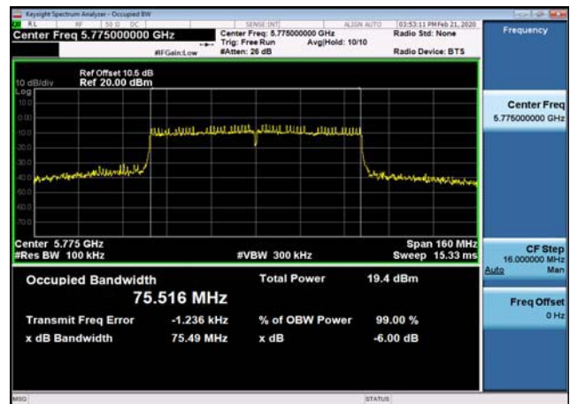
U-NII-3 6dB Bandwidth-802.11ac(80MHz) ,5775MHz,Ant1
