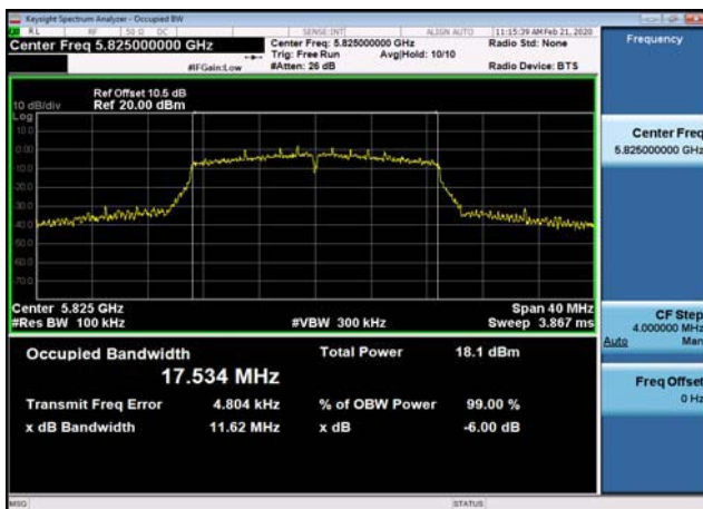
U-NII-3 6dB Bandwidth-802.11ac(40MHz) ,5795MHz,Ant1
