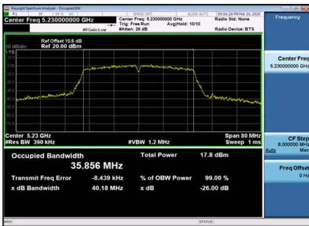
U-NII-3 6dB Bandwidth-802.11n(20MHz),5745MHz,Ant1
