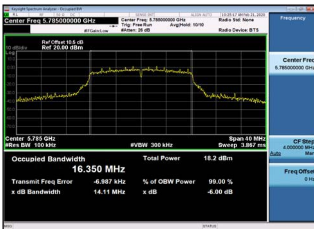
U-NII-3 6dB Bandwidth-802.11ac(20MHz) ,5745MHz,Ant1
