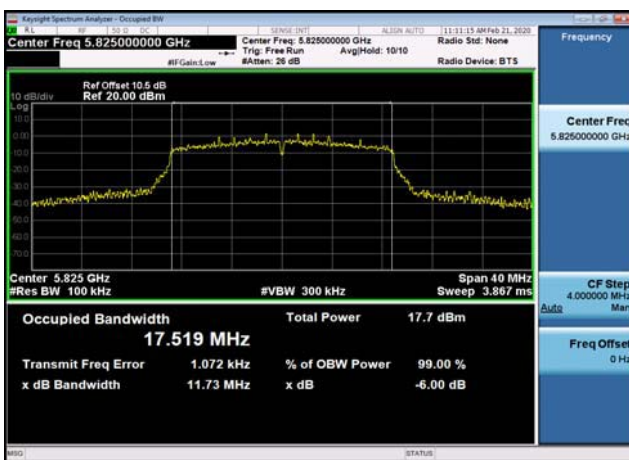
U-NII-3 6dB Bandwidth-802.11n(20MHz),5825MHz,Ant1
