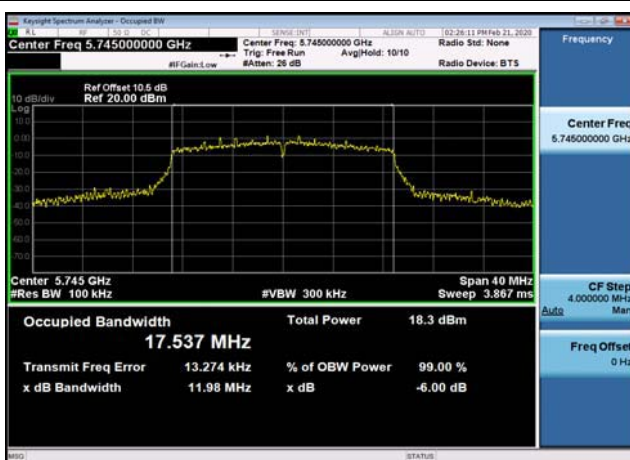
U-NII-3 6dB Bandwidth-802.11ac(20MHz) ,5745MHz,Ant1
