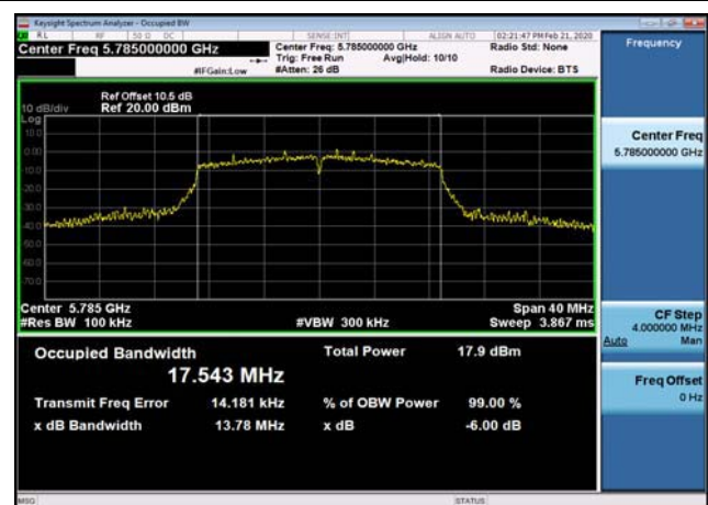
U-NII-3 6dB Bandwidth-802.11ac(20MHz) ,5785MHz,Ant1
