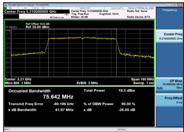
U-NII-3 6dB Bandwidth-802.11n(20MHz),5785MHz,Ant1
