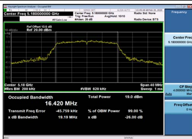
U-NII-1 26dB Bandwidth-802.11a(20MHz) ,5180MHz
