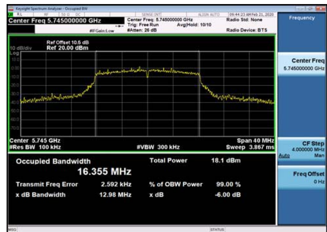
U-NII-3 6dB Bandwidth-802.11a(20MHz) ,5825MHz,Ant1
