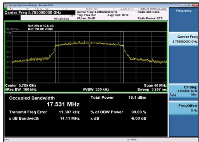
U-NII-3 6dB Bandwidth-802.11n(40MHz),5755MHz,Ant1
