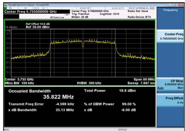
U-NII-3 6dB Bandwidth-802.11ac(80MHz) ,5775MHz,Ant1
