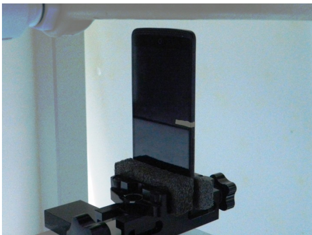
Bottom Side, Test Separation 10 mm
