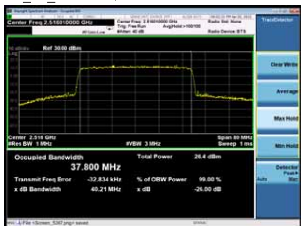
DC_2A_n41A 64QAM 100 %RB 40MHz CH-Low
