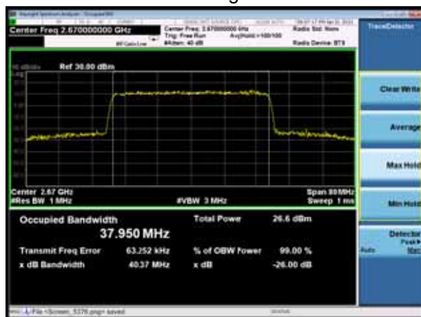
DC_2A_n41A 256QAM 100 %RB 40MHz CH-High
