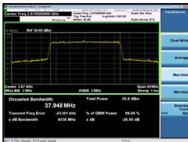
DC_2A_n41A 16QAM 100 %RB 40MHz CH-High
