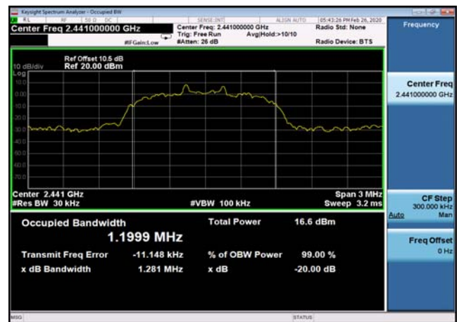
20dB Bandwidth: 8DPSK,2441MHz,3DH5
