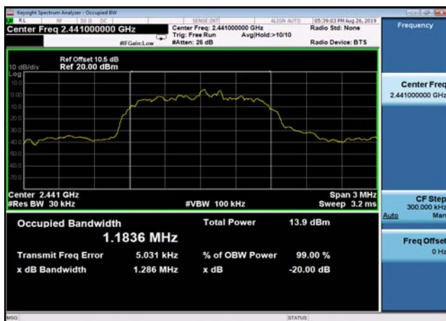
20dB Bandwidth: DQPSK,2441MHz,2DH5
