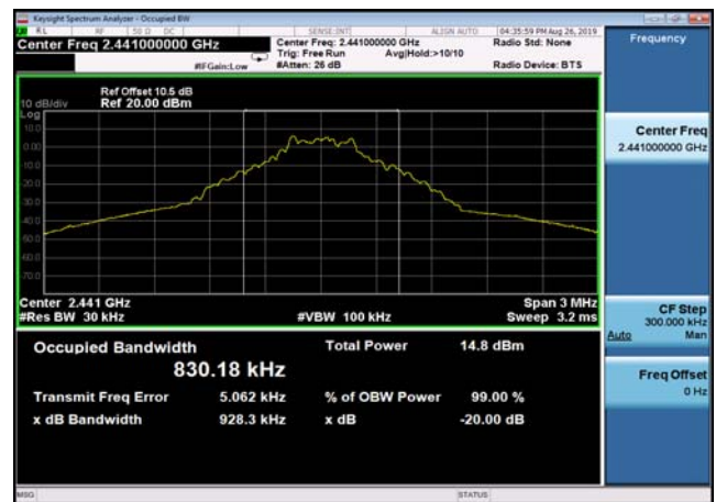
20dB Bandwidth: DQPSK,2402MHz,2DH5
