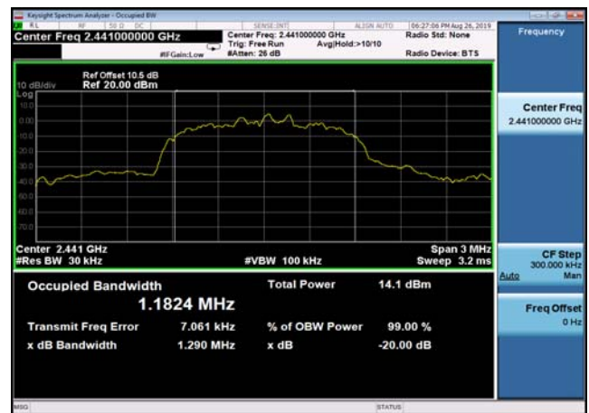
20dB Bandwidth: 8DPSK,2441MHz,3DH5
