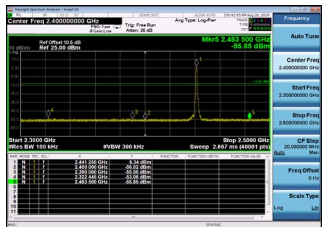
Conducted Emission: DQPSK,2441,2DH5 ,Band Edge HoppingOFF
