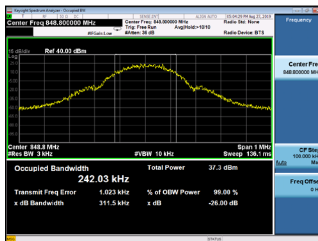
(Plot A3: GSM 850MHz Channel = 251 Occupied bandwidth)
