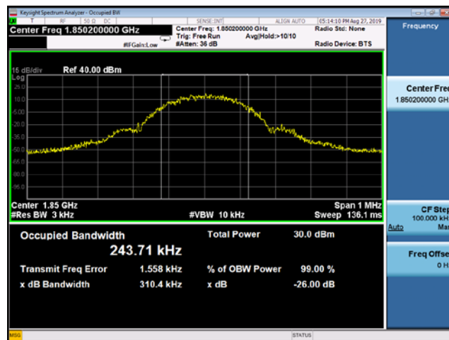
(Plot D1: EDGE 1900MHz Channel = 512 Occupied bandwidth)
