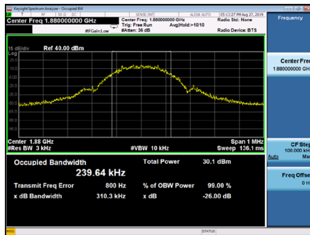
(Plot D2: EDGE 1900MHz Channel = 661 Occupied bandwidth)
