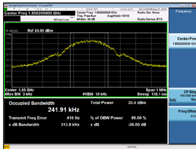
(Plot B1: GSM 1900MHz Channel = 512 Occupied bandwidth)
