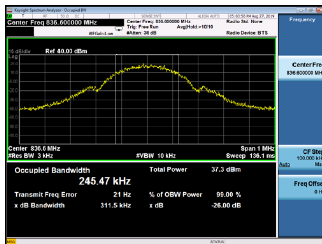
(Plot A2: GSM 850MHz Channel = 190 Occupied bandwidth)
