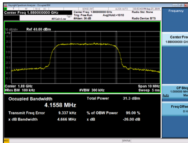
(Plot F2: WCDMA 1900MHz Channel = 9400 Occupied bandwidth)
