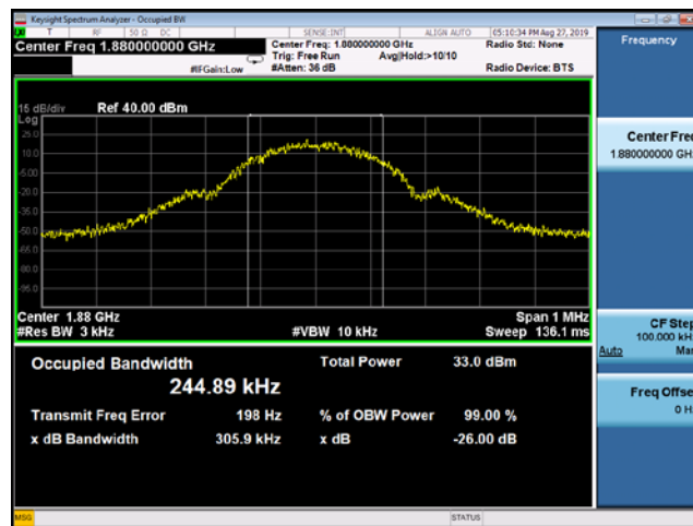
(Plot B2: GSM 1900MHz Channel = 661 Occupied bandwidth)
