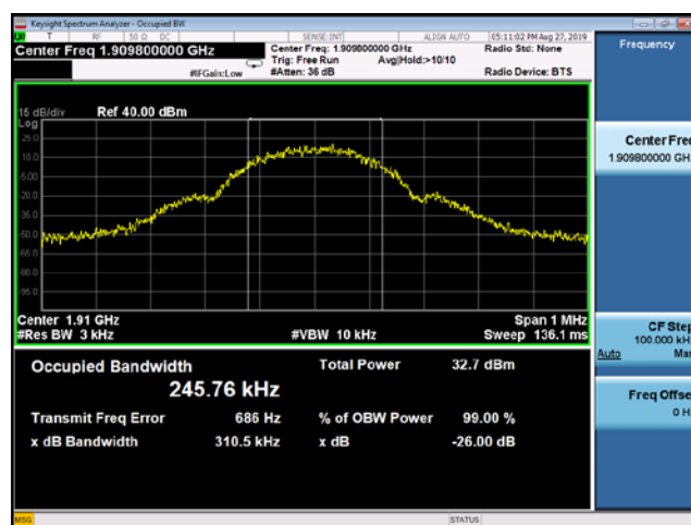
(Plot B3: GSM 1900MHz Channel = 810 Occupied bandwidth)
