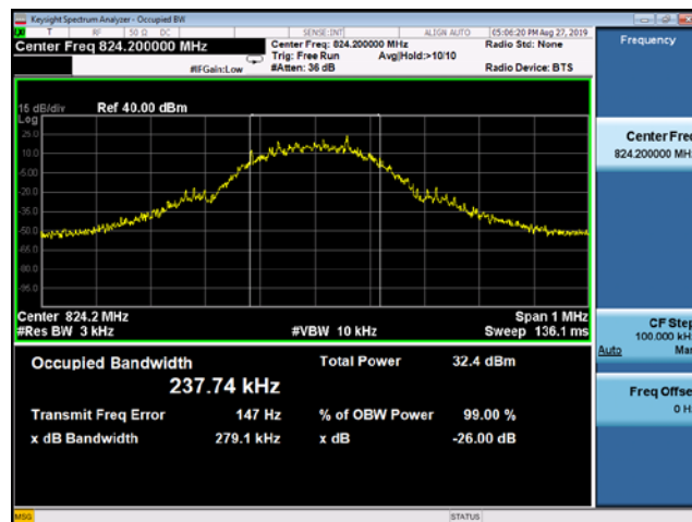
(Plot C1: EDGE 850MHz Channel = 128 Occupied bandwidth)
