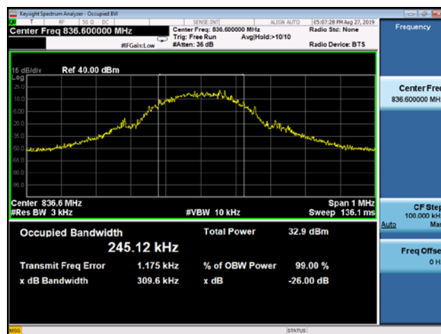
(Plot C2: EDGE 850MHz Channel = 190 Occupied bandwidth)
