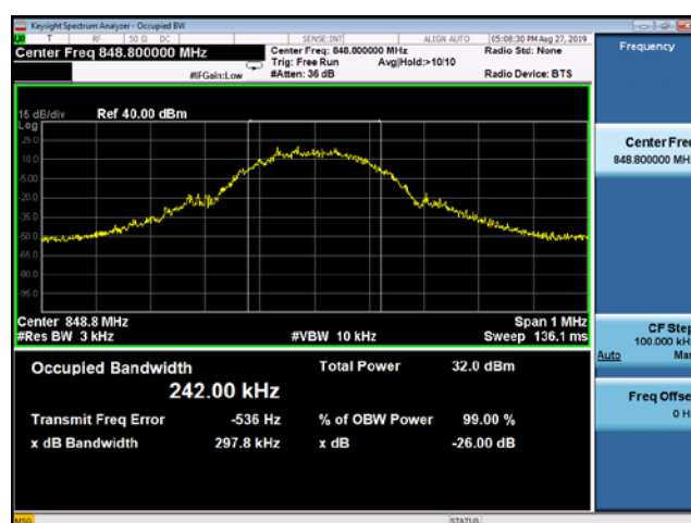
(Plot C3: EDGE 850MHz Channel = 251 Occupied bandwidth)
