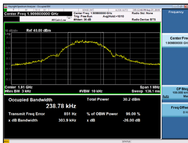
(Plot D3: EDGE 1900MHz Channel = 810 Occupied bandwidth)
