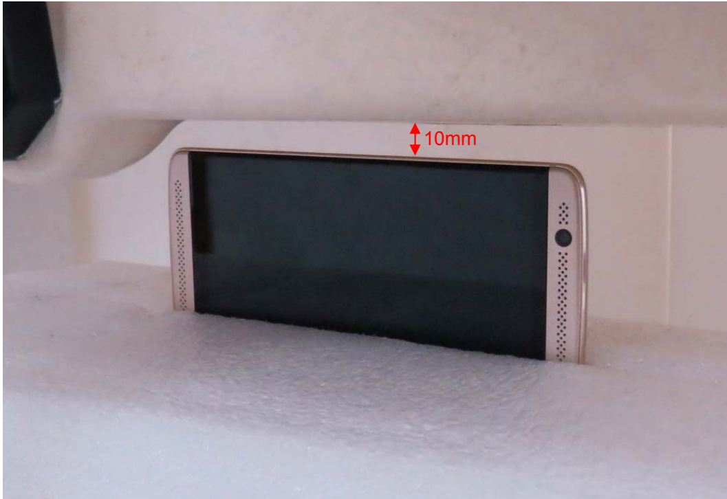
Picture 22: Left Side, the distance from handset to the bottom of the Phantom is 10mm
