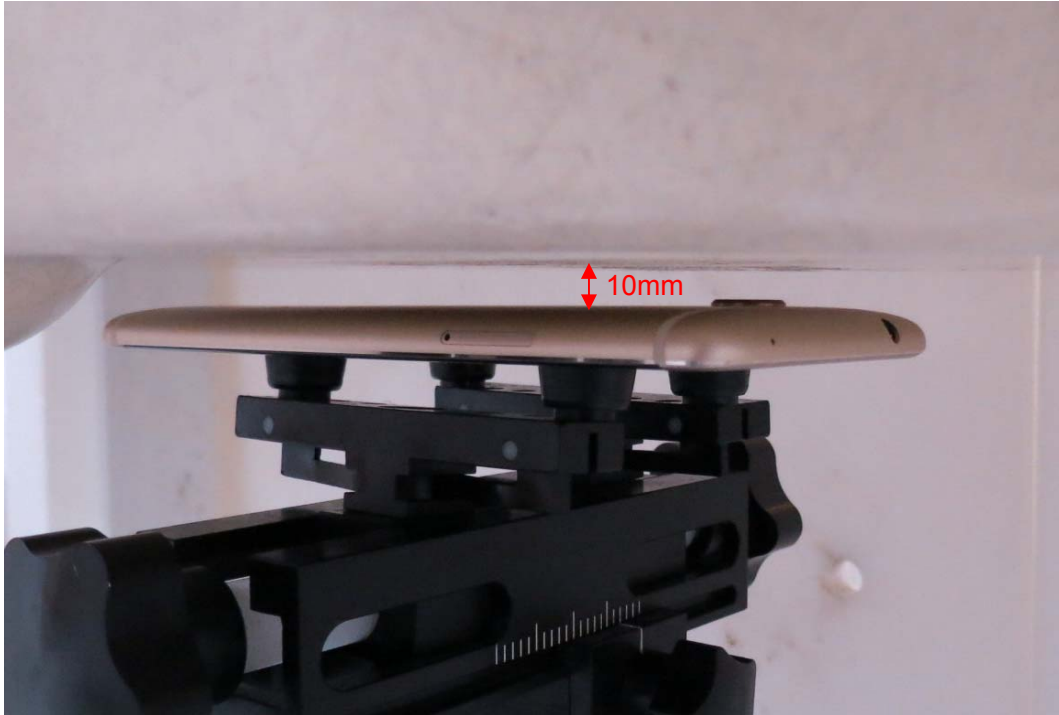
Picture 20: Back Side, the distance from handset to the bottom of the Phantom is 10mm
