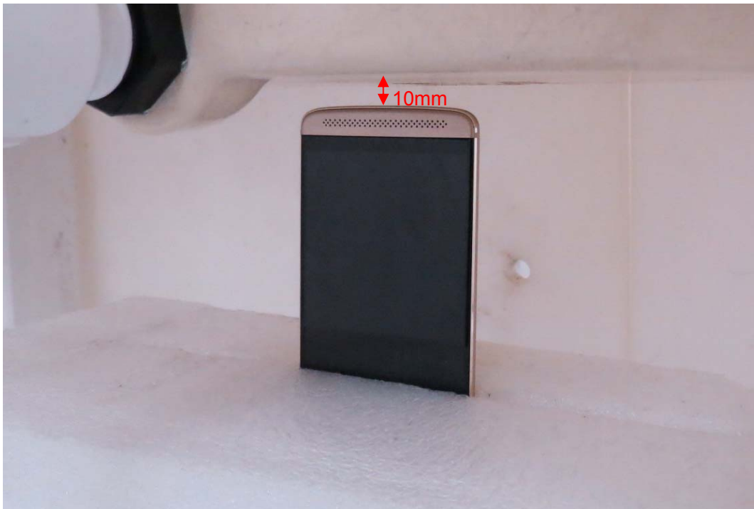
Picture 25: Bottom Side, the distance from handset to the bottom of the Phantom is 10mm
