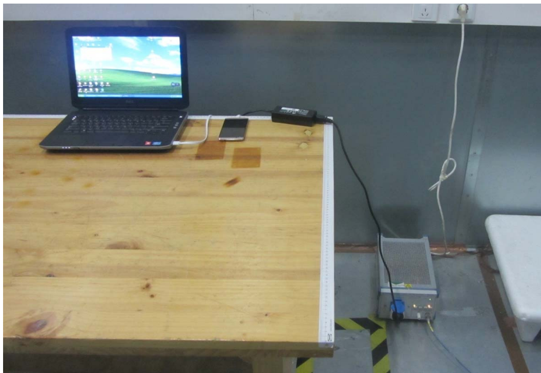
Picture 3 Conducted Emission Test Setup
