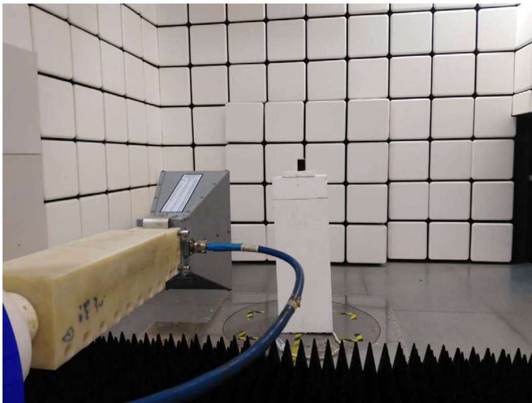
Picture 2: Radiated Spurious Emissions Test setup
