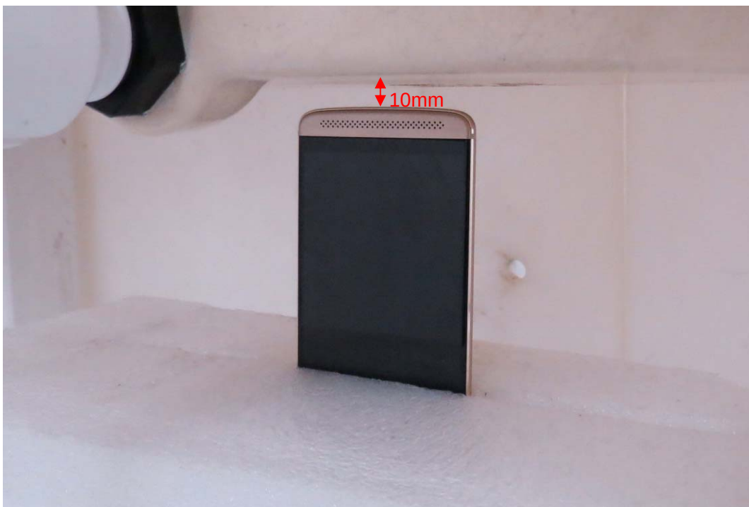
Bottom Side, the distance from handset to the bottom of the Phantom is 10mm
