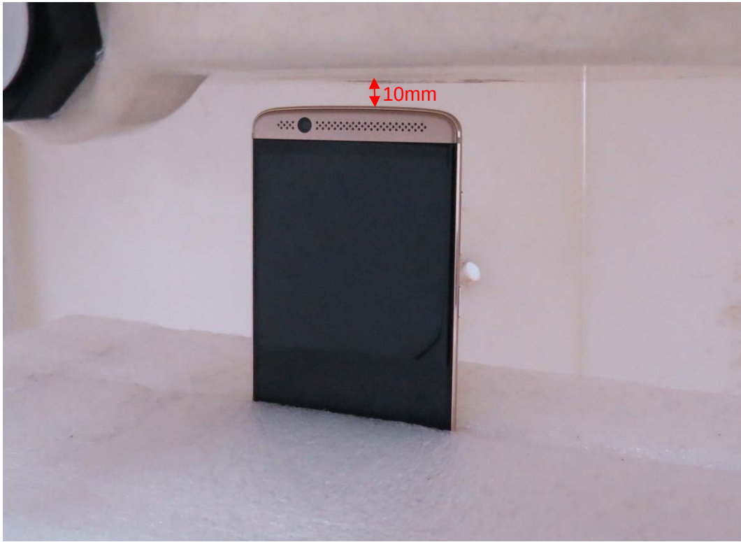
Top Side, the distance from handset to the bottom of the Phantom is 10mm
