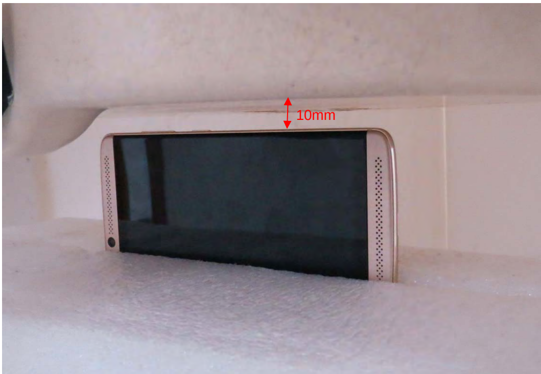
Picture 28: Right Side, the distance from handset to the bottom of the Phantom is 10mm (Original)
