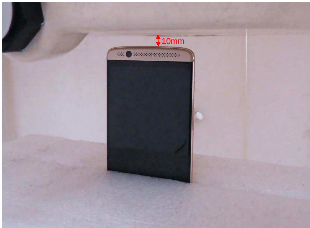
Picture 29: Top Side, the distance from handset to the bottom of the Phantom is 10mm (Original)
