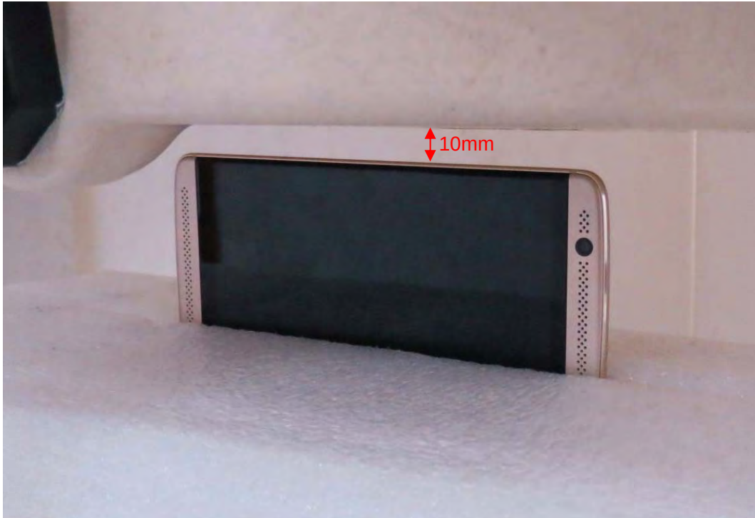
Picture 27: Left Side, the distance from handset to the bottom of the Phantom is 10mm (Original)
