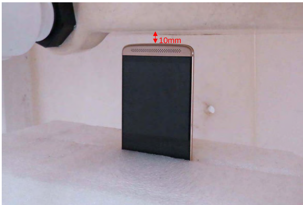
Picture 30: Bottom Side, the distance from handset to the bottom of the Phantom is 10mm (Original)
