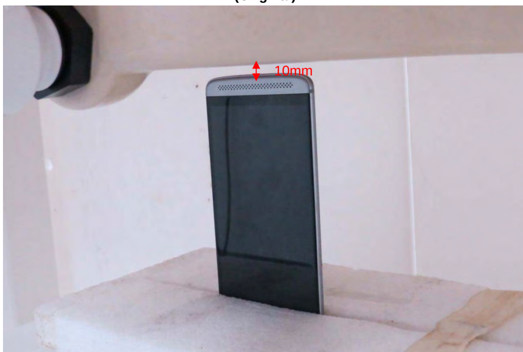
Picture 31: Bottom Side, the distance from handset to the bottom of the Phantom is 10mm (Variant)
