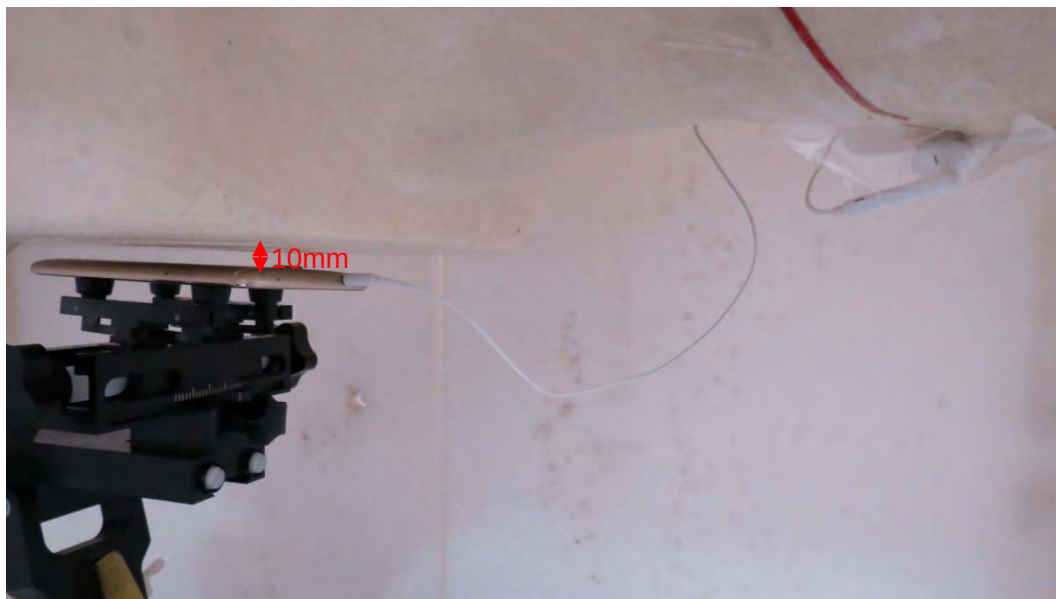
Picture 32: Back Side with Earphone, the distance from handset to the bottom of the Phantom is 10mm (Original)
