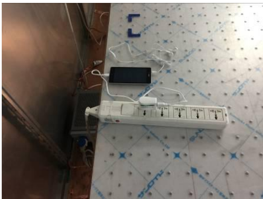
Pic9: Conducted Emissions Test Setup (with charger)
