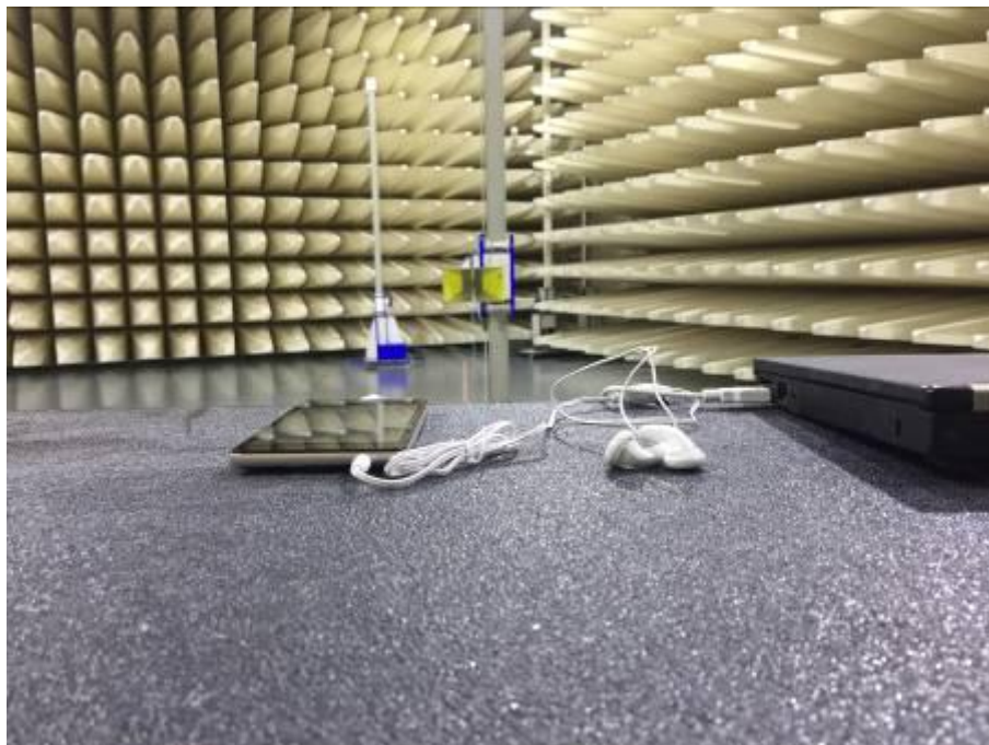
Pic6: Radiated Emissions Test Setup (with laptop)
