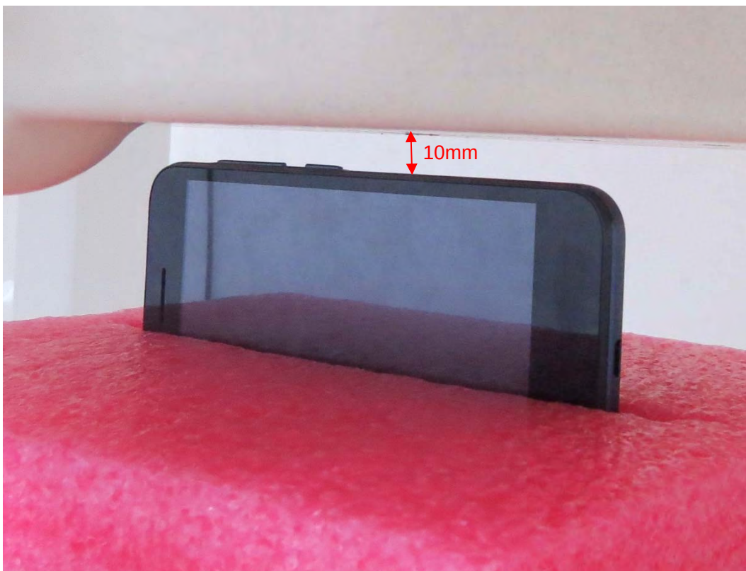
Picture 23: Right Side, the distance from handset to the bottom of the Phantom is 10mm
