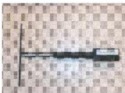
Figure 1 – Satimo COMOSAR Validation Dipole
