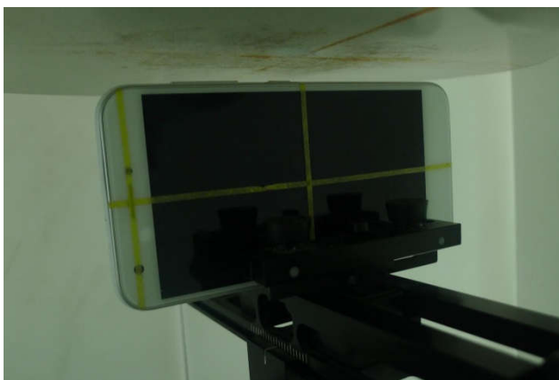
Right Side, Test Separation 10 mm
