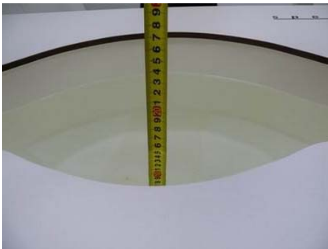
Picture 8: Liquid depth in the flat Phantom (1900 MHz, 15.2cm depth)
