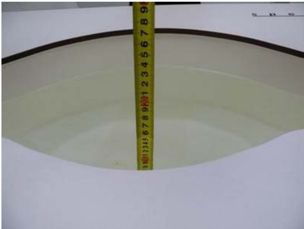
Picture 6: Liquid depth in the flat Phantom (1750 MHz, 15.2cm depth)
