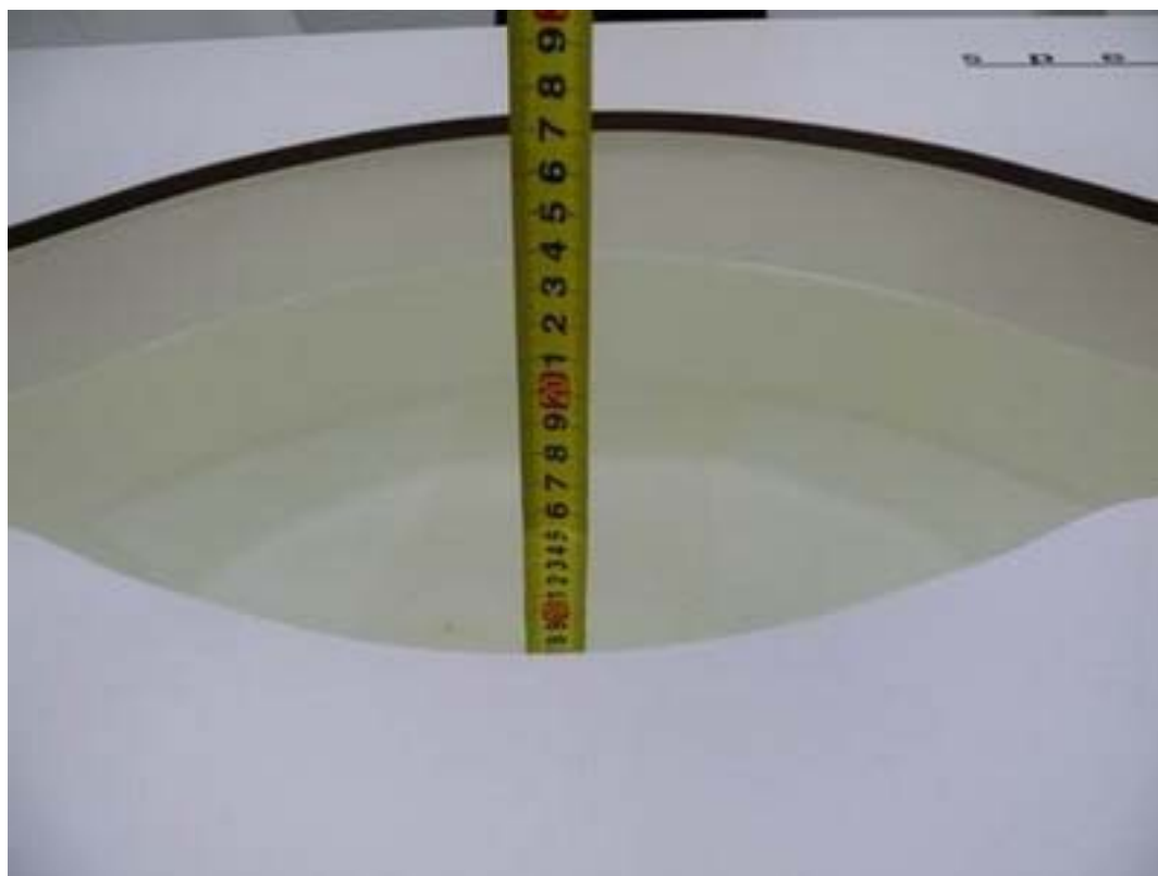
Picture 8: Liquid depth in the flat Phantom (1750 MHz, 15.2cm depth)
