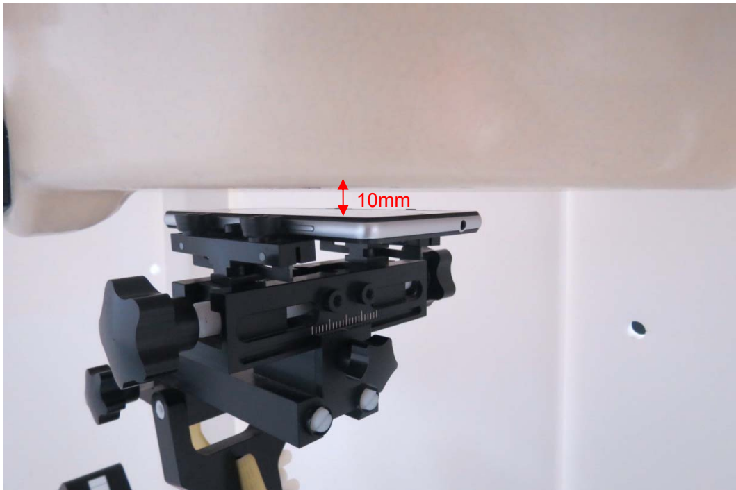
Picture 21: Front Side, the distance from handset to the bottom of the Phantom is 10mm
